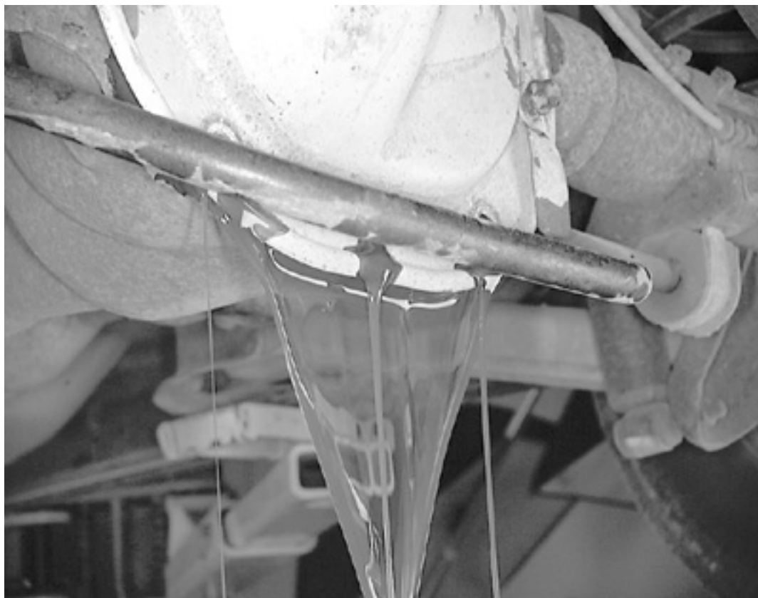
After the cover bolts are removed, carefully pry the cover loose so that fluid begins to drain from the bottom
