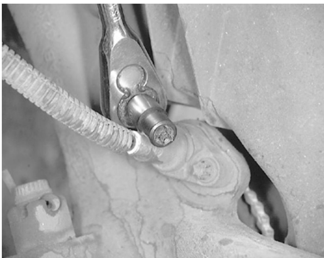
A special E6 Torx® socket is required to remove the speed sensor retaining bolt
