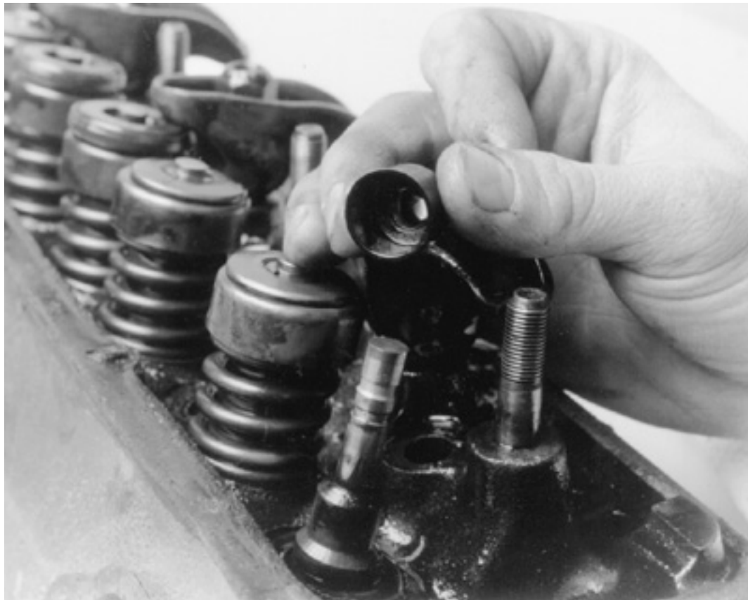
Removing an umbrella/positive type seal
