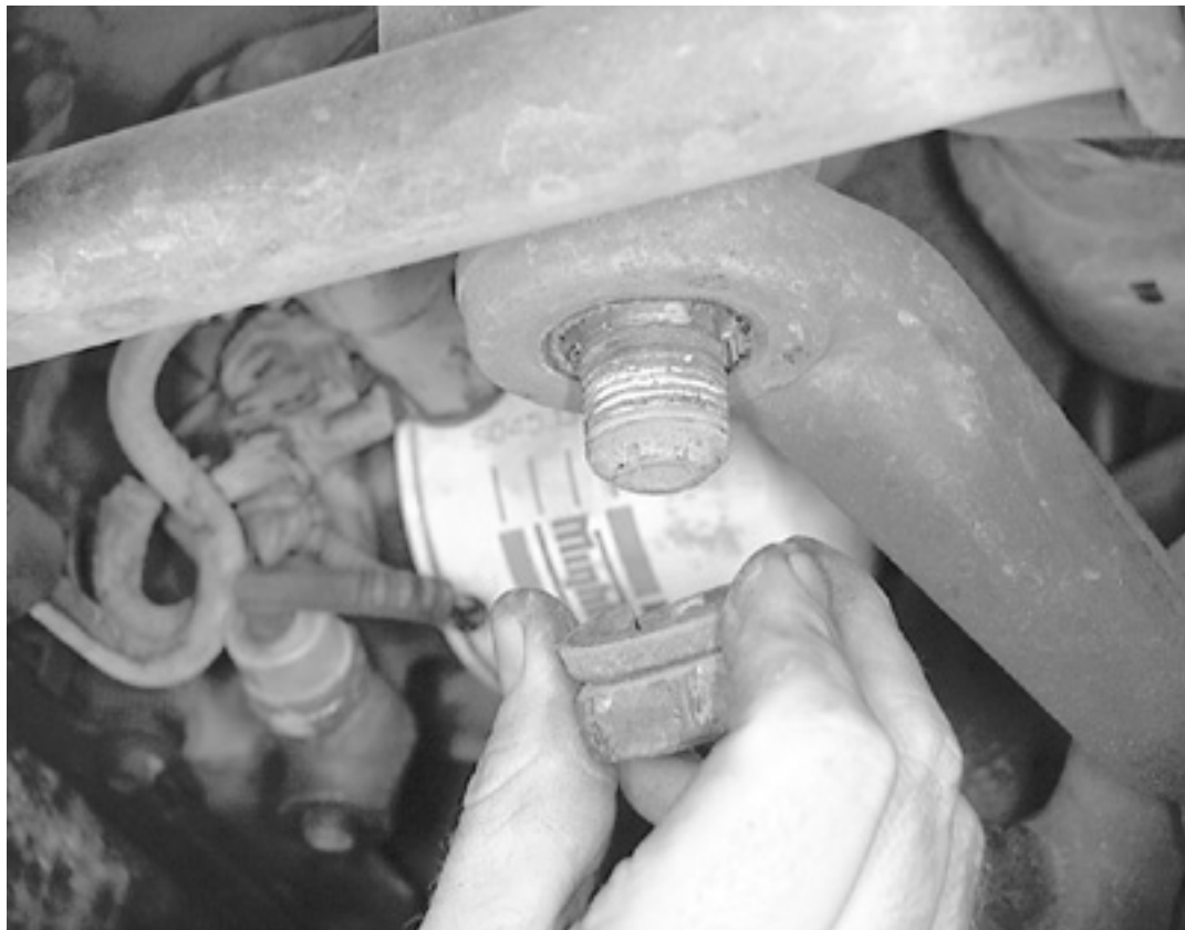
Remove the pitman arm retaining nut and lockwasher
