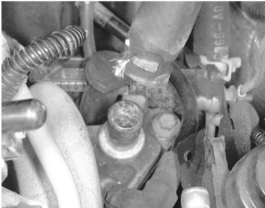
Remove the heater hoses from the intake manifold
