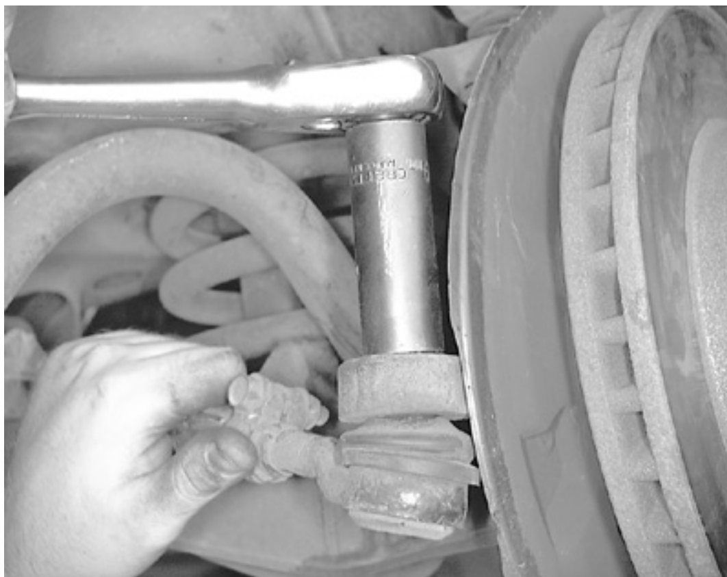
Remove the tie rod end-to-steering knuckle retaining nut
