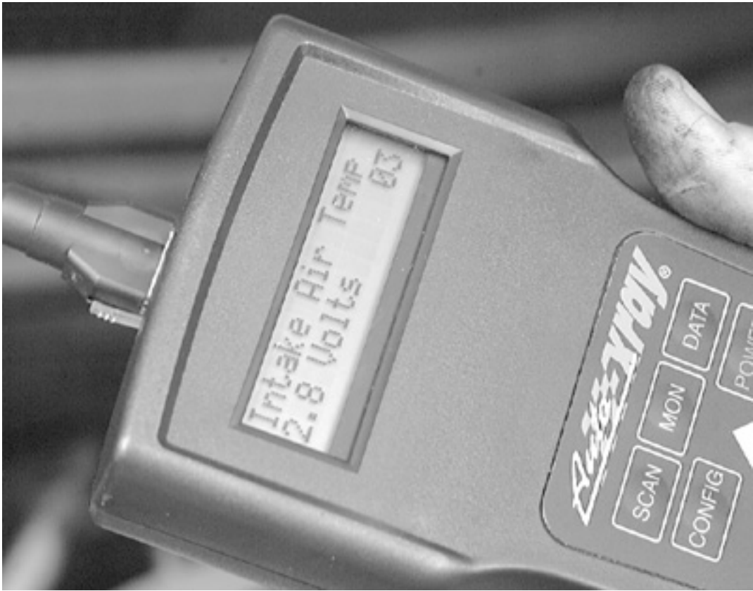
The IAT sensor can be monitored with an appropriate and Data-stream capable scan tool
