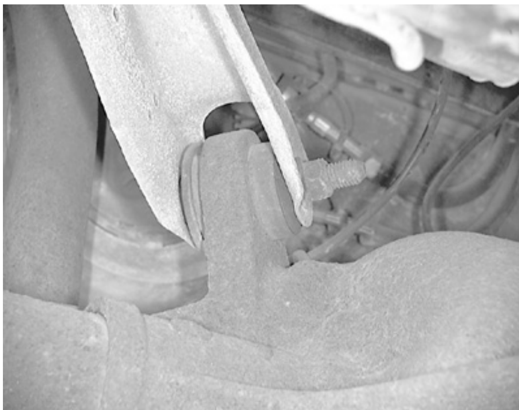
Upper control arm-to-axle mounting
