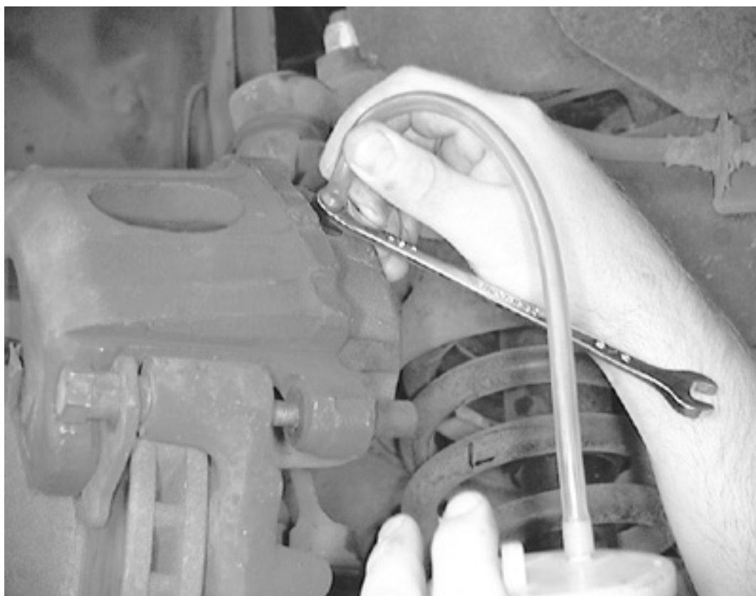
Attach a length of rubber hose over the bleeder screw and place the other end of the hose in a glass jar
