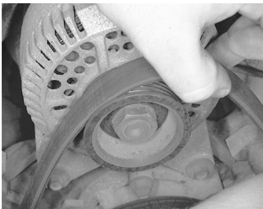
Rotate the tensioner and remove the belt from around the alternator pulley
