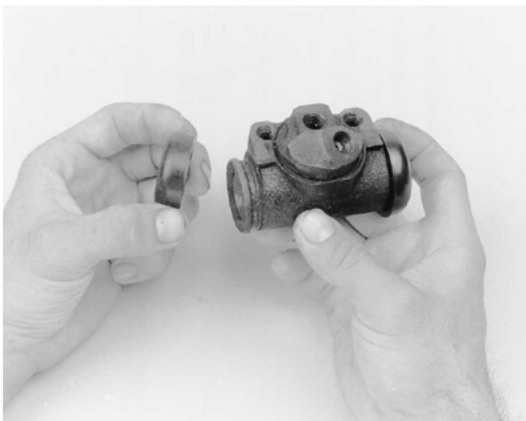
The boots can now be installed over the wheel cylinder ends
