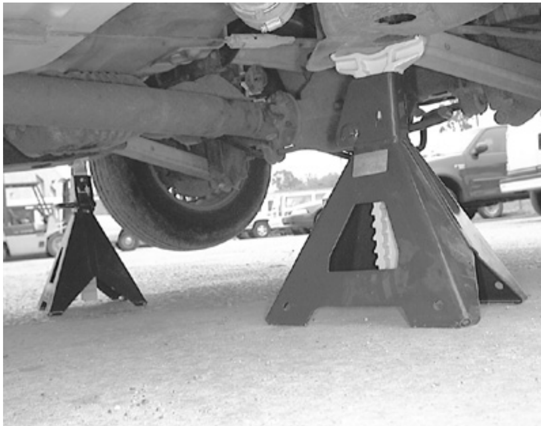
Locate the jackstands under the frame as shown to support the rear of the vehicle
