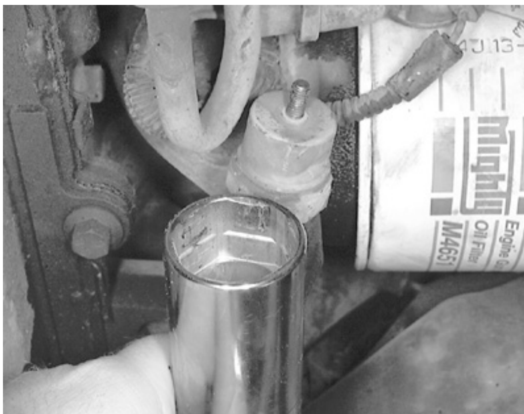
A special socket is available to remove the sender/switch
