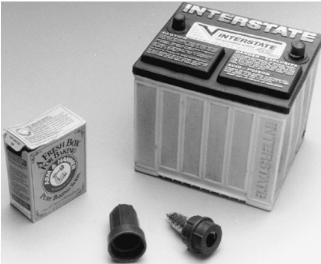
Maintenance is performed with household items and with special tools like this post cleaner
