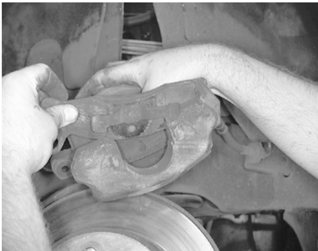
Removing the outer brake pad
