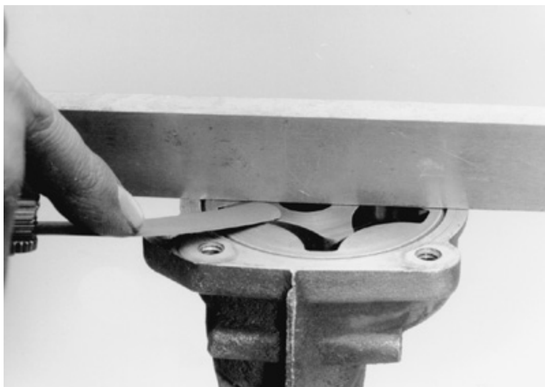
Measuring oil pump rotor end-play—5.0L and 5.8L engines
