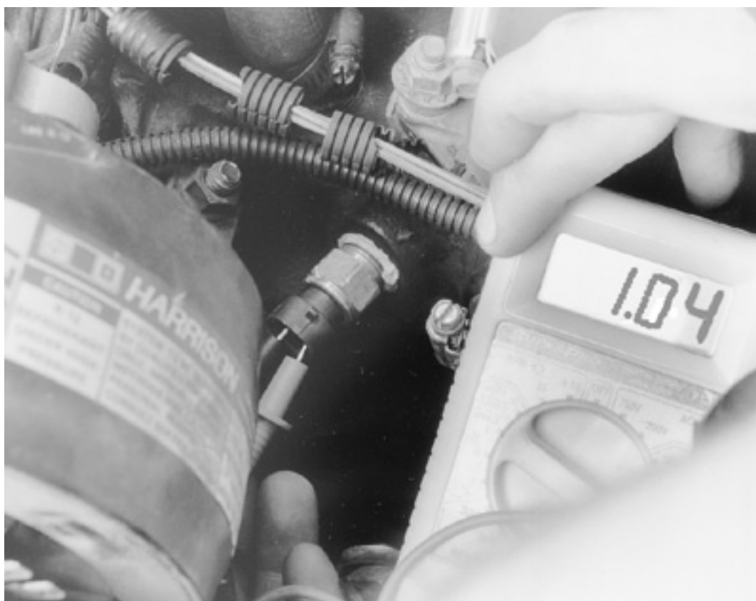
Checking the resistance of a coolant temperature sensor with an ohmmeter. Reading is 1.04 kilohms
