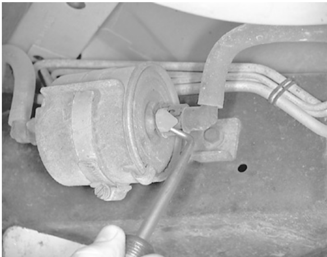
Release the clips holding the fuel lines to the filter by gently prying them from the line. A cotter pin puller works very well for this
