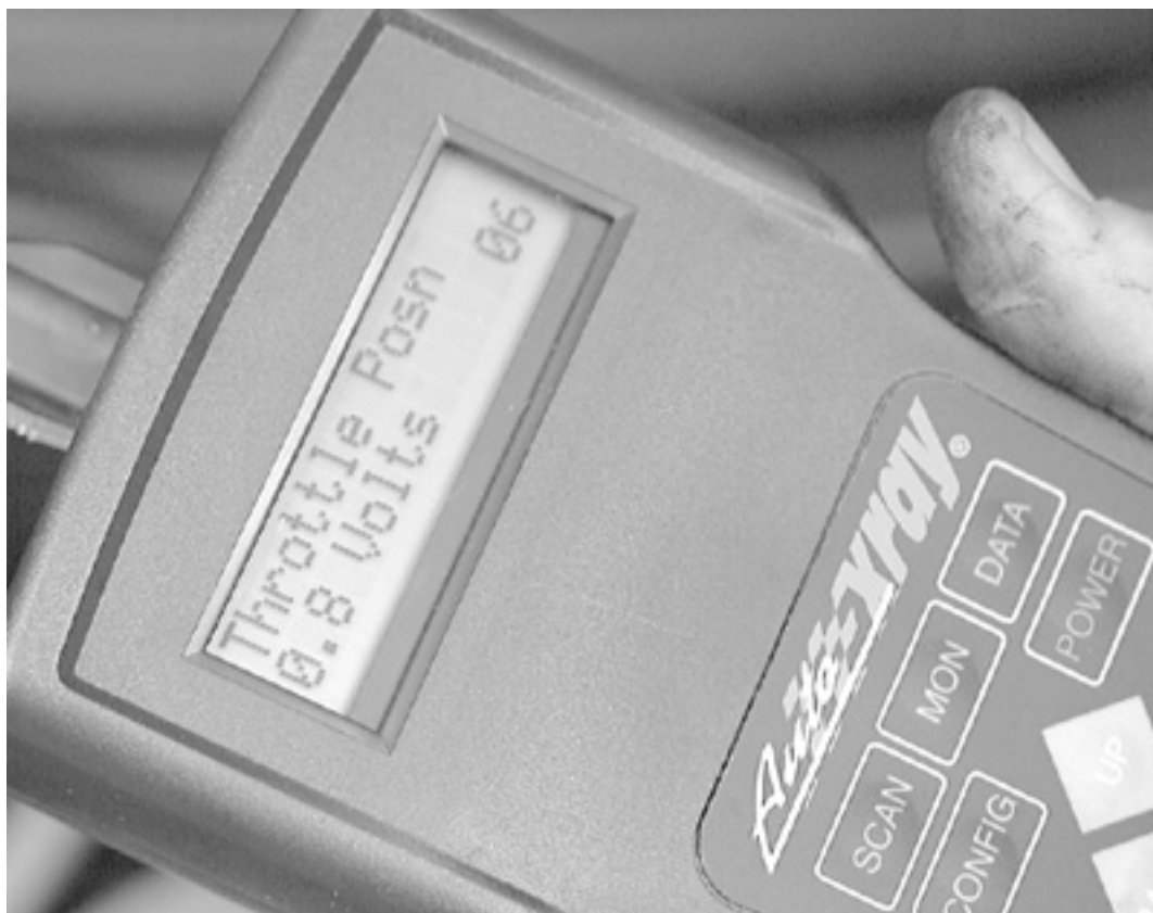
The TP sensor can be monitored with an appropriate and Data-stream capable scan tool
