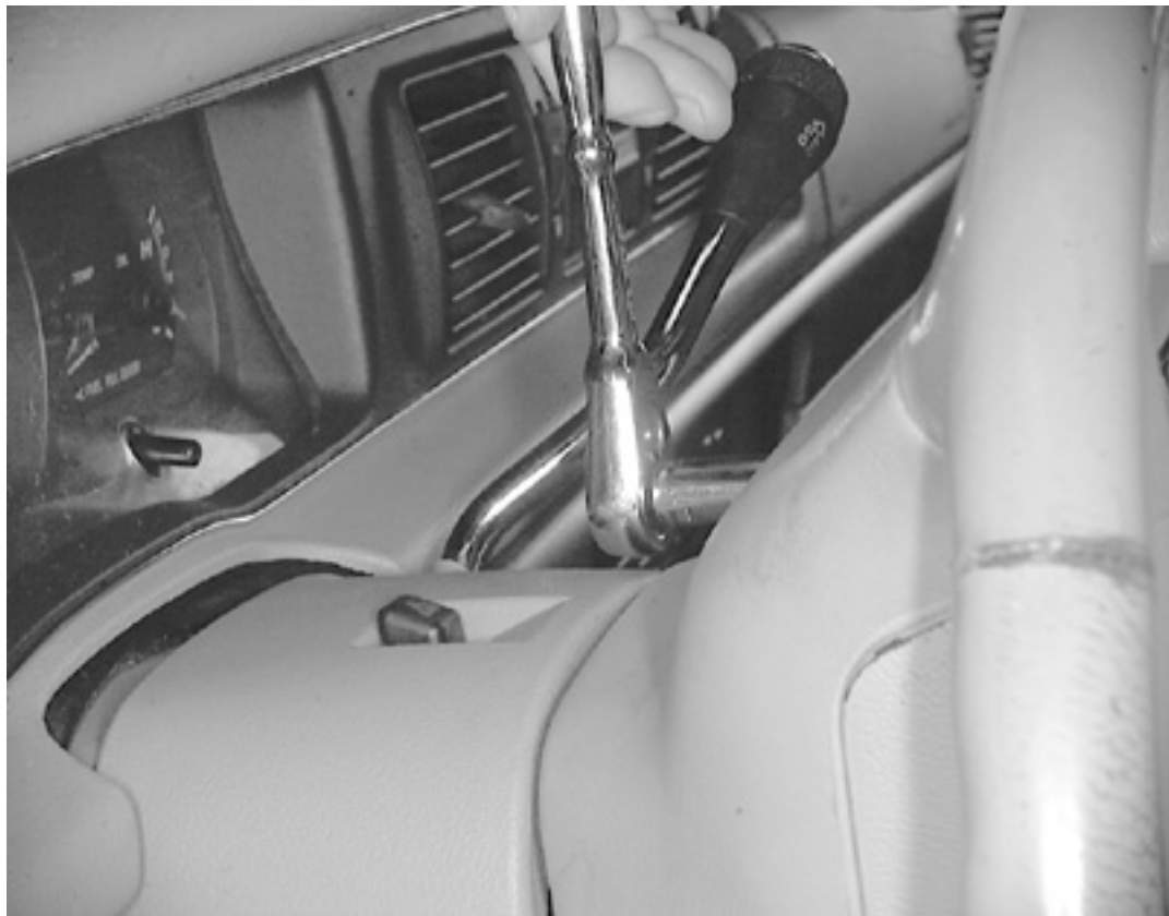
Remove the air bag module retaining bolts
