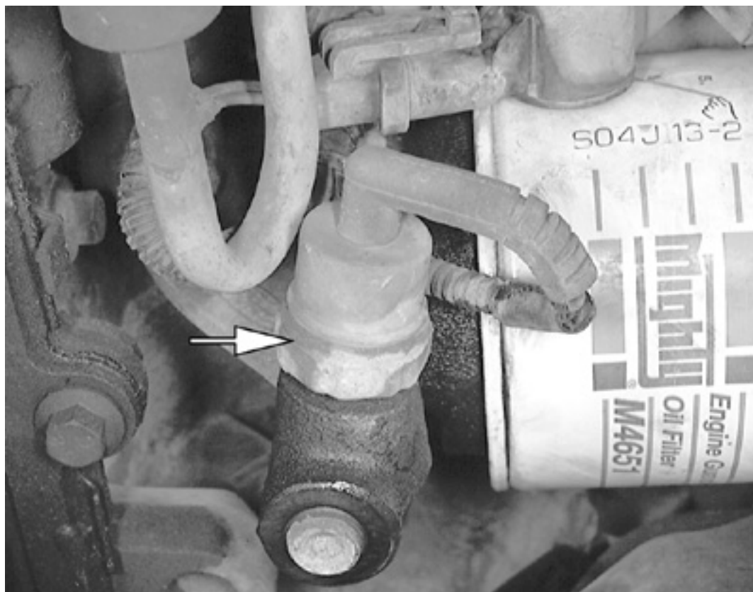
Oil pressure sender/switch—4.6L engine
