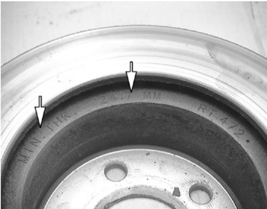
On the front rotor, the minimum thickness specification is usually stamped on the inside edge
