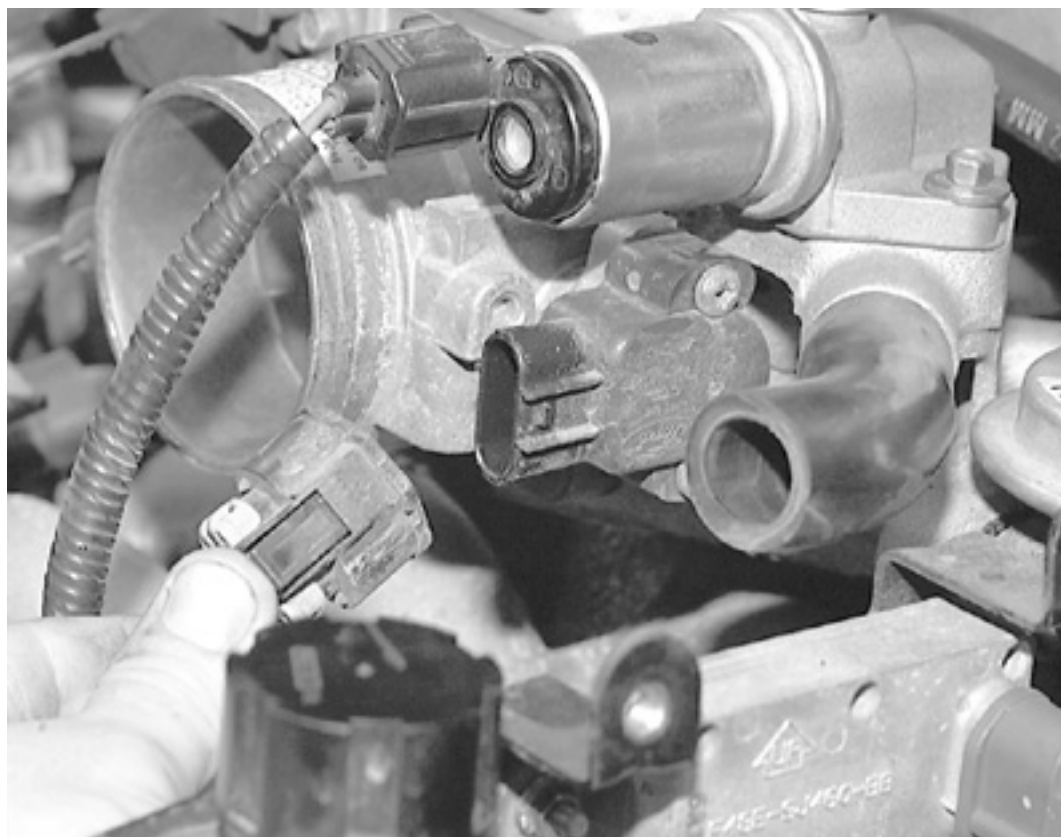
Detach the TP sensor connector
