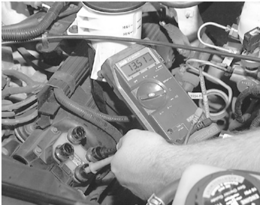
Testing the secondary ignition coil resistance-4.6L engine
