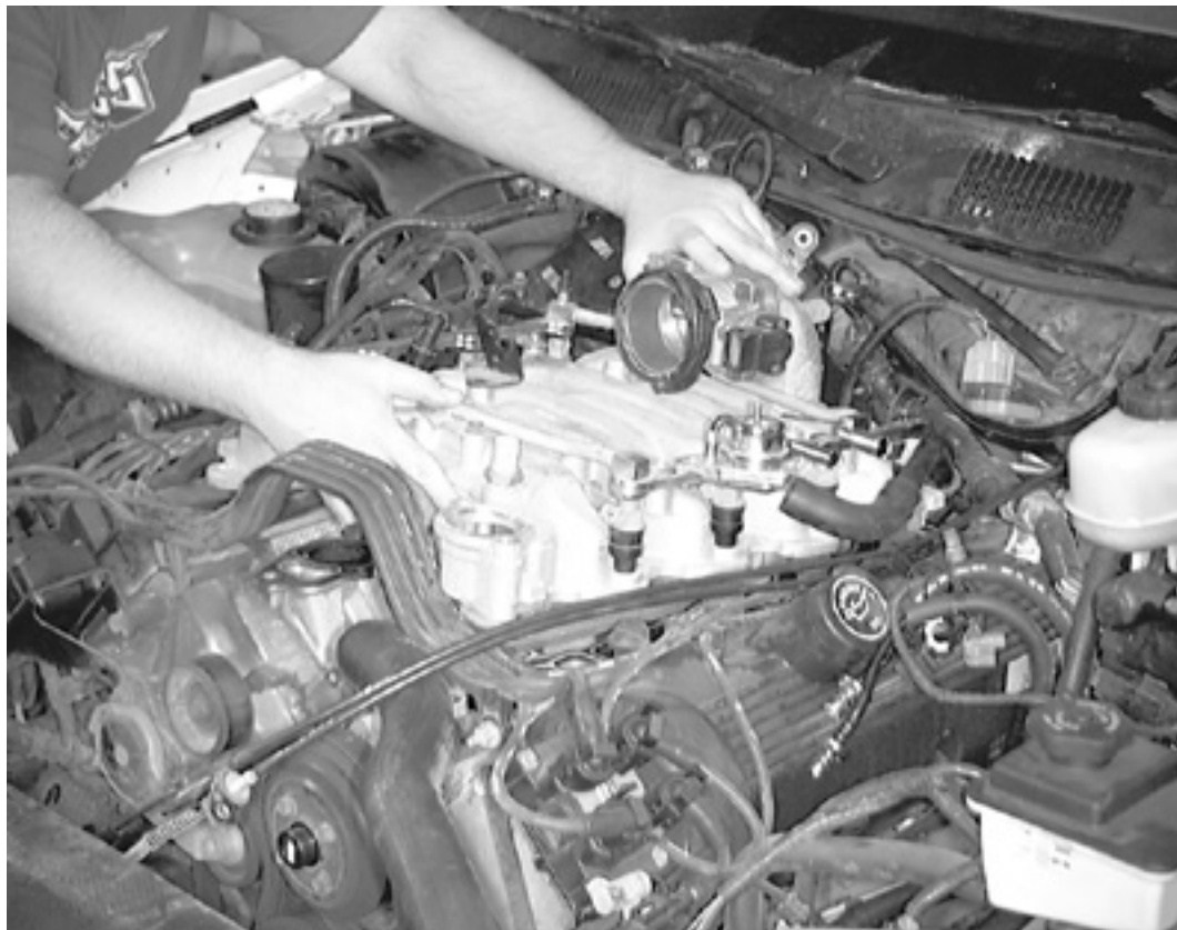
Carefully lift the intake manifold from the engine
