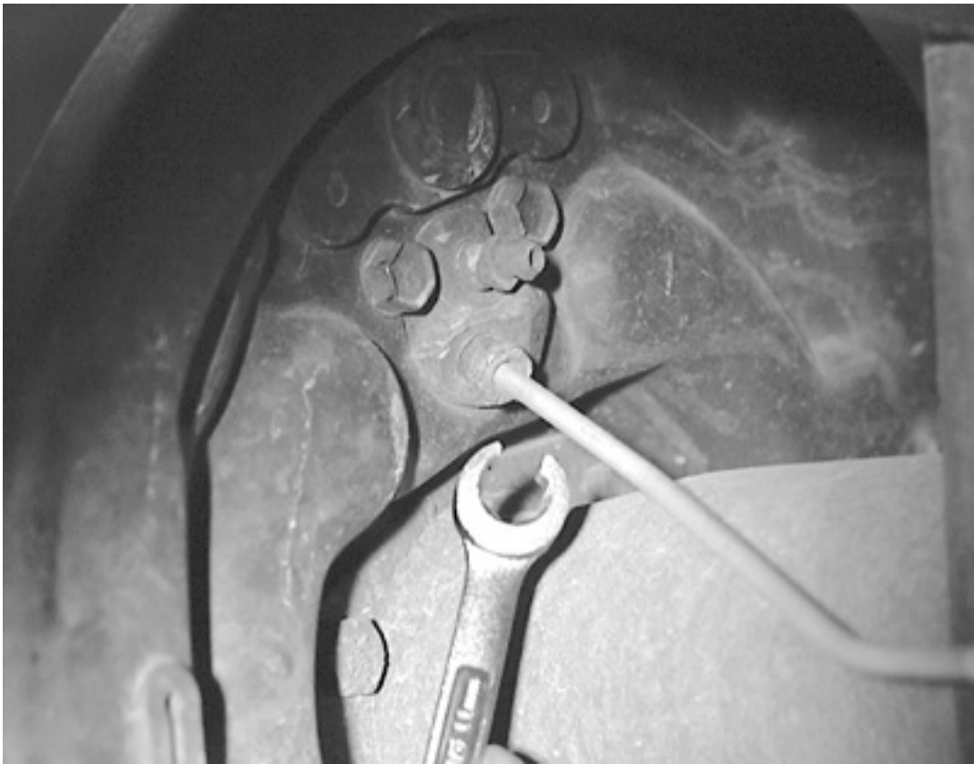
Use a suitable size flare nut wrench to ...
