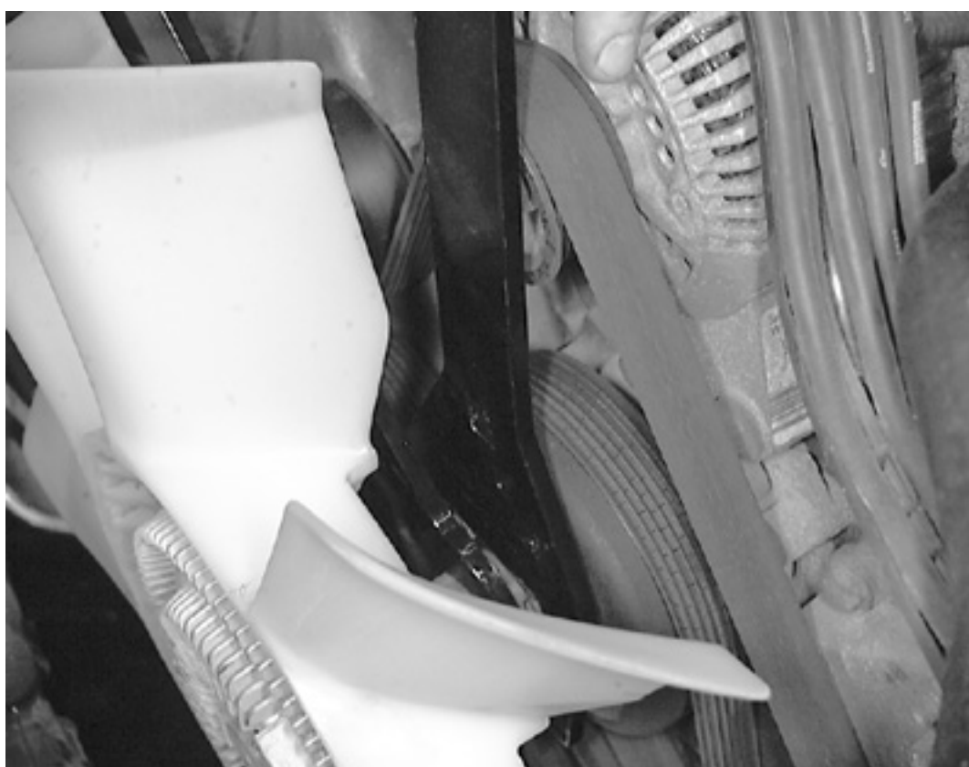
Place the special fan removal tools over the water pump pulley bolts and onto the fan clutch hub and loosen the fan clutch assembly
