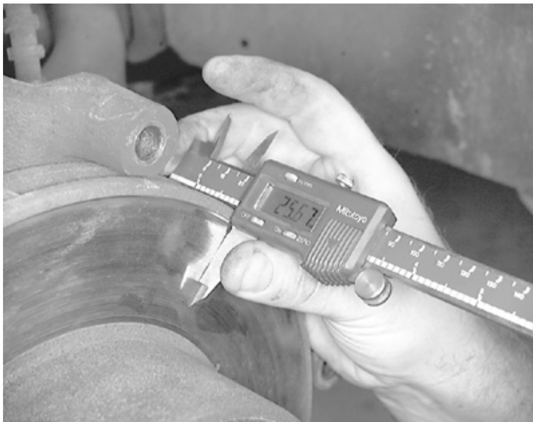
Check brake rotor thickness in several places around the rotor using a Vernier caliper
