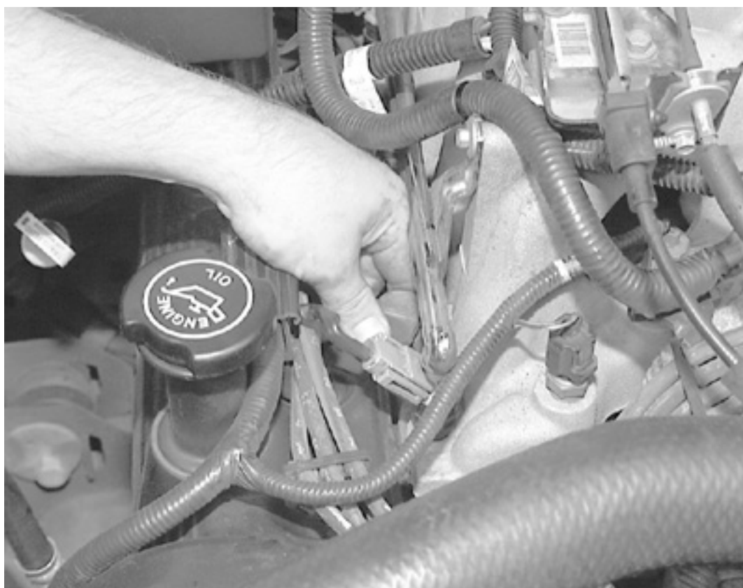
Grasp the plug wire and carefully twist the wire to release the retainer from the spark plug
