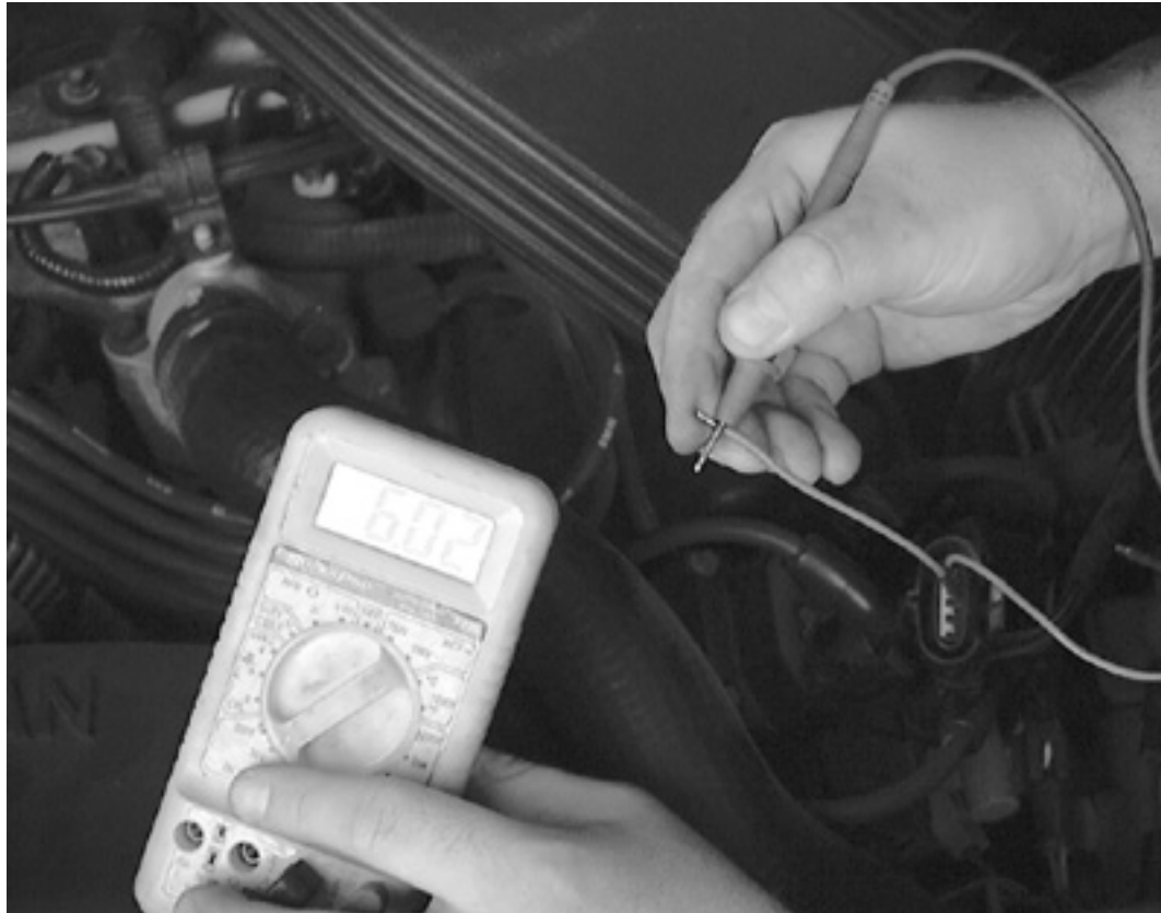
Testing the SIG circuit of the MAF sensor
