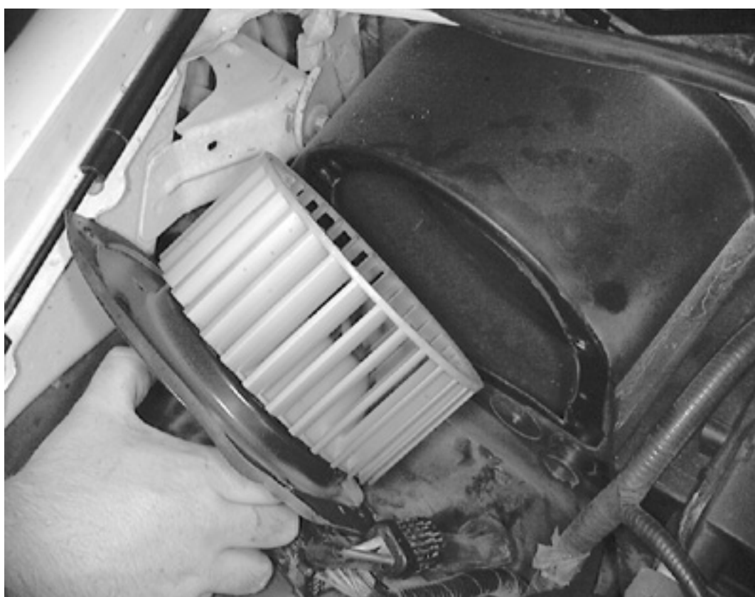
Turn the blower motor and wheel assembly slightly to the right so the bottom edge of the mounting plate follows the contour of the wheel well splash panel to remove it from the vehicle
