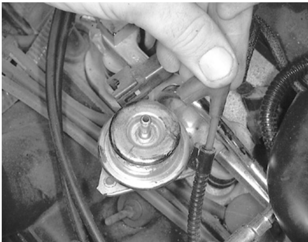
Disconnect the vacuum hoses from the fuel pressure regulator and ...
