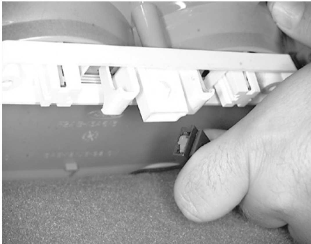
Detach the connector for the high mount brake lamp
