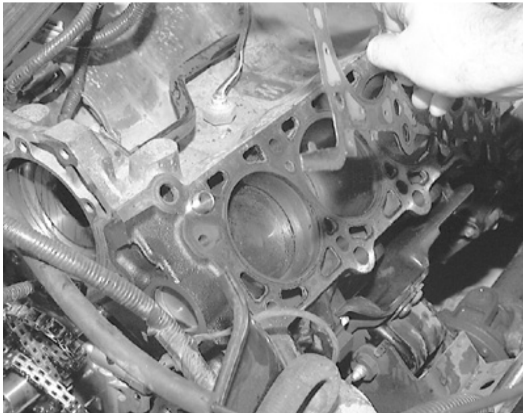
Remove the head gasket from the engine block
