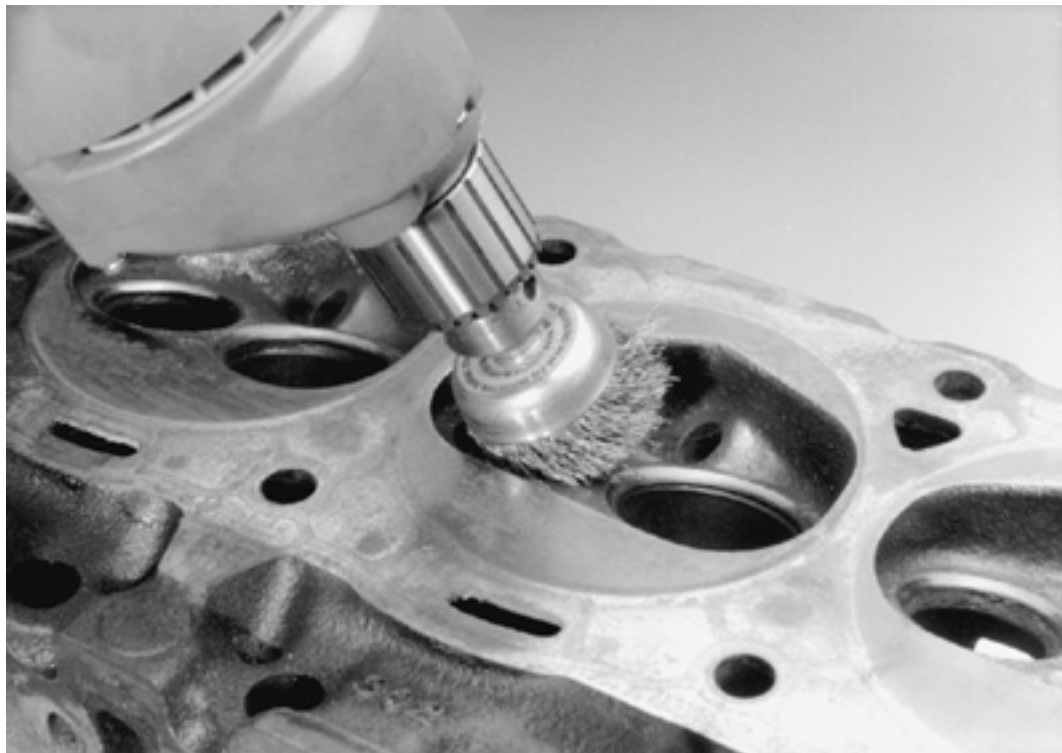
Cleaning the combustion chamber with drill-mounted wire brush—5.0L engine shown
