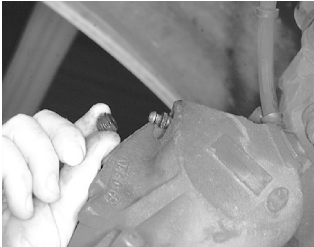
Remove the bleeder screw rubber dust cover—front caliper
