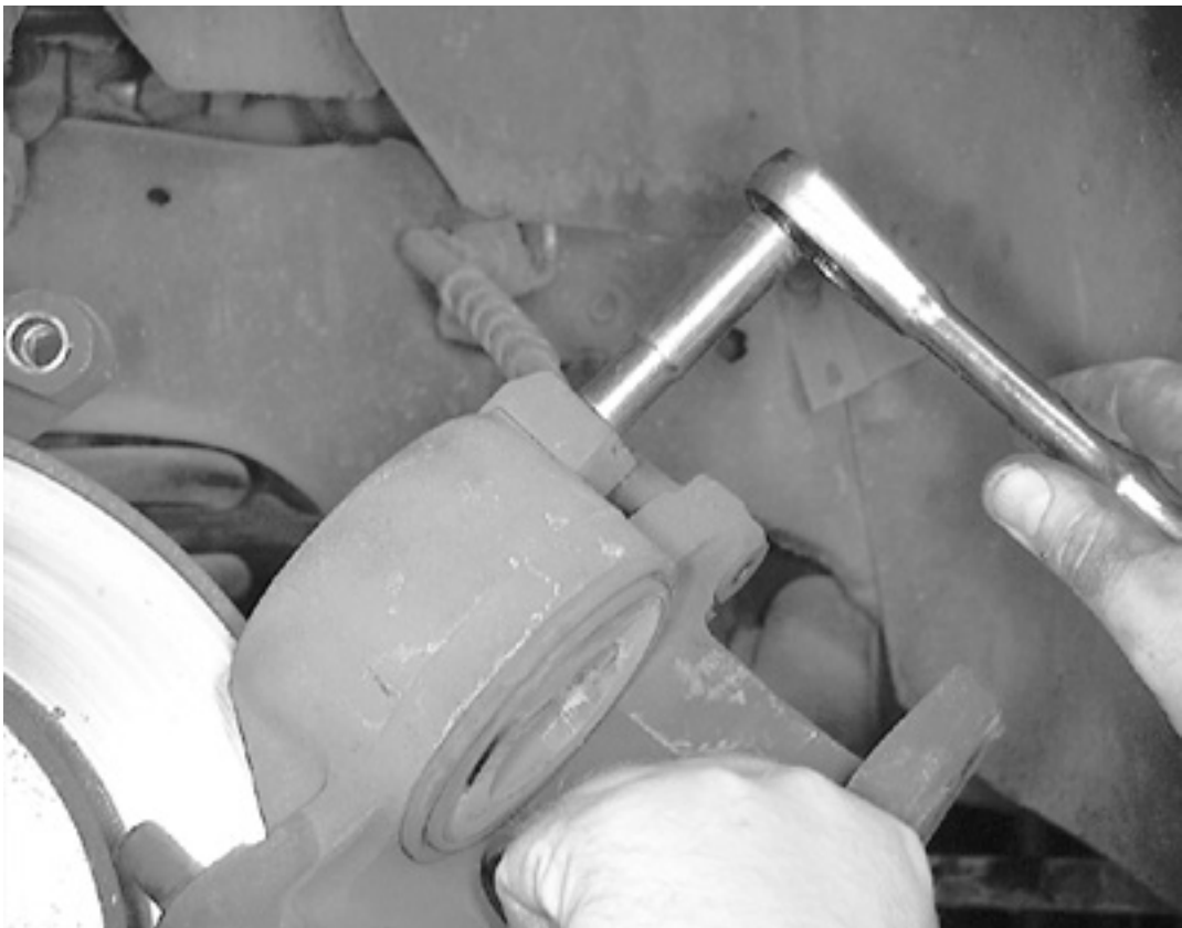
Remove the front brake hose banjo bolt and ...
