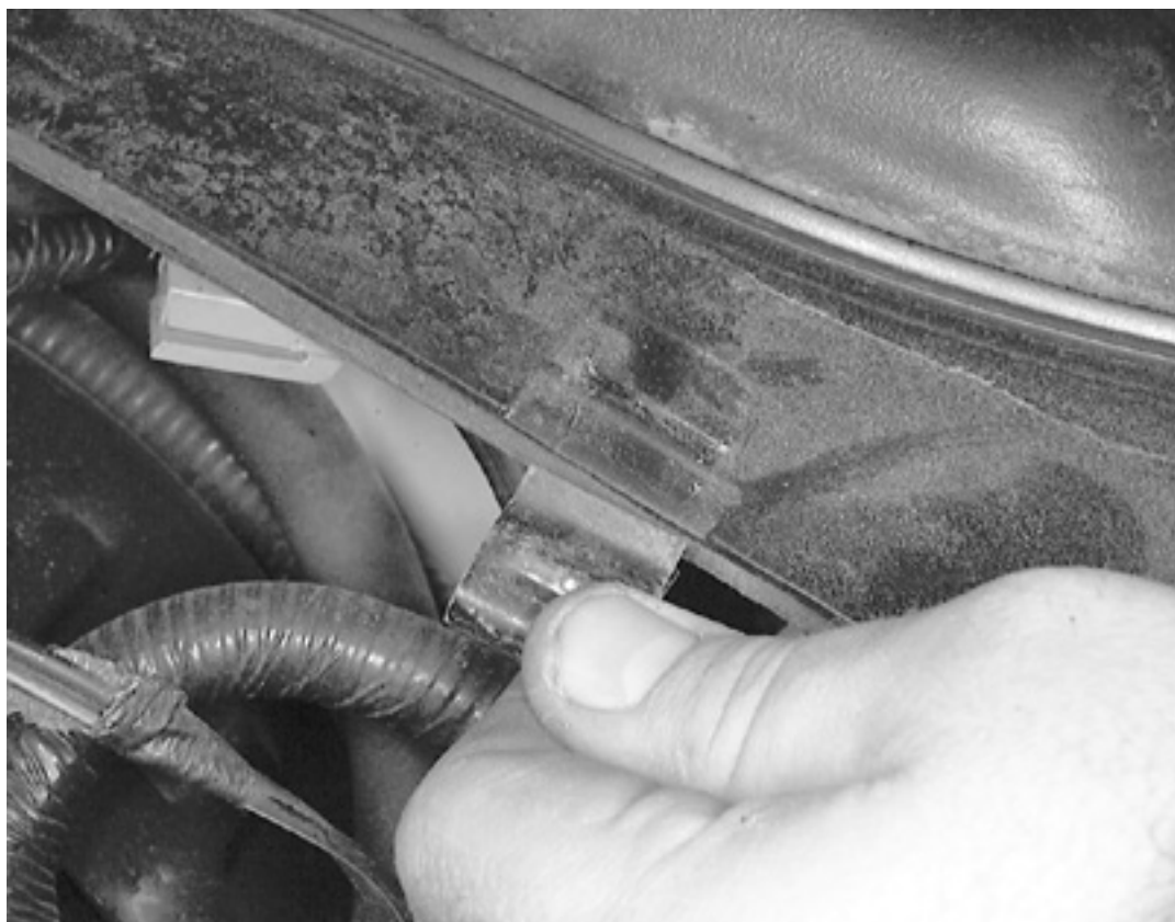
Remove the cowl panel-to-firewall retaining clips
