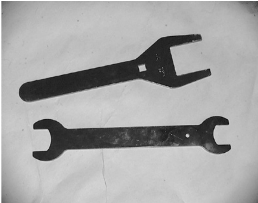
Special wrenches to remove the fan clutch assembly like these are available from manufacturers such as Lisle®
