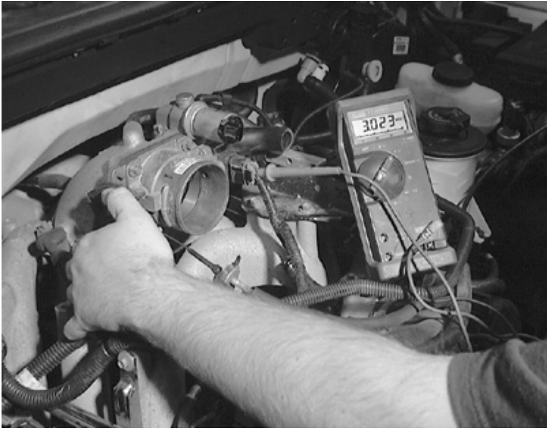
Test the operation of the TP sensor by gently opening the throttle while observing the signal return voltage. The voltage should move smoothly according to the amount the throttle is opened
