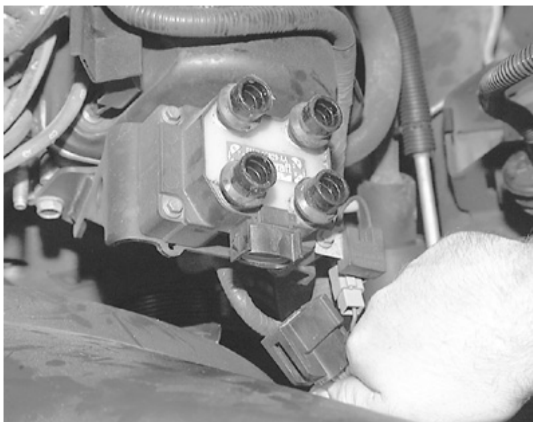
Detach the connector for the coil pack
