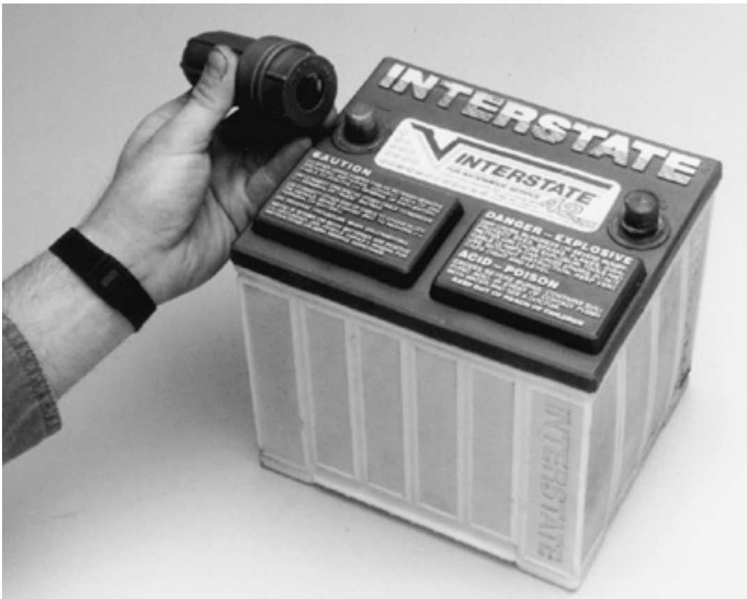
The underside of this special battery tool has a wire brush to clean post terminals
