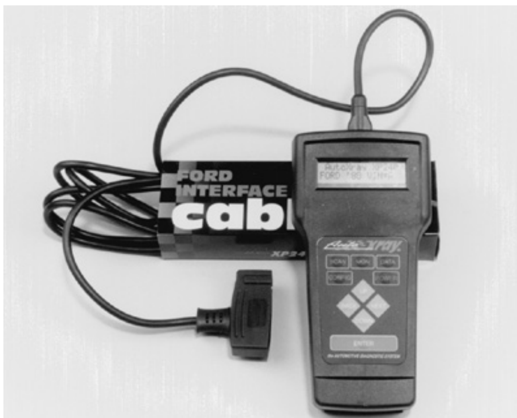
Inexpensive scan tools, such as this Auto Xray®, are available to interface with your Ford vehicle
