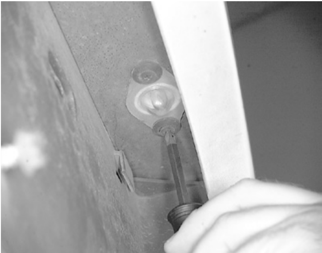
Use a Phillips head screwdriver to remove the 2 plastic rivets retaining the light assembly to the rear bumper
