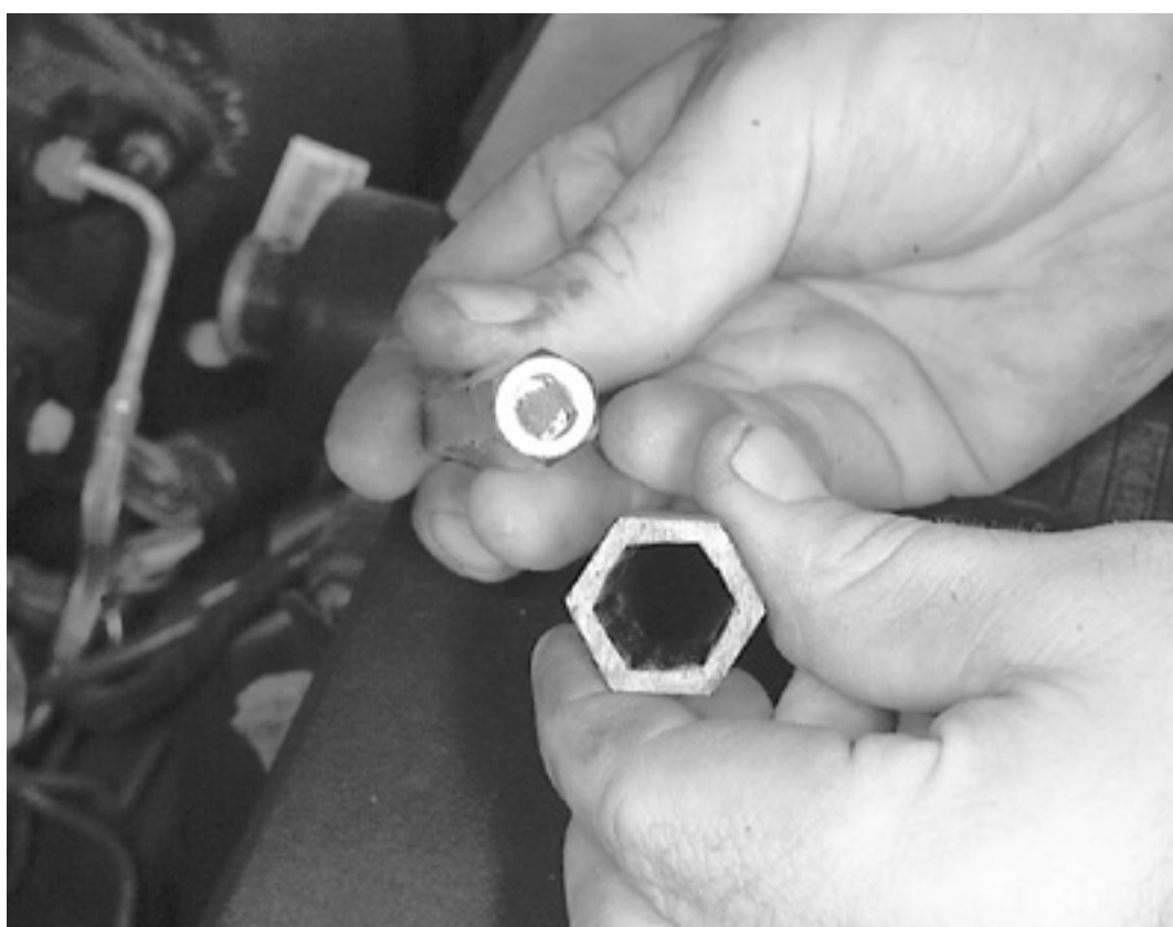
Special tools, such as these from Lisle®, are extremely helpful in removing the upper mounting nut
