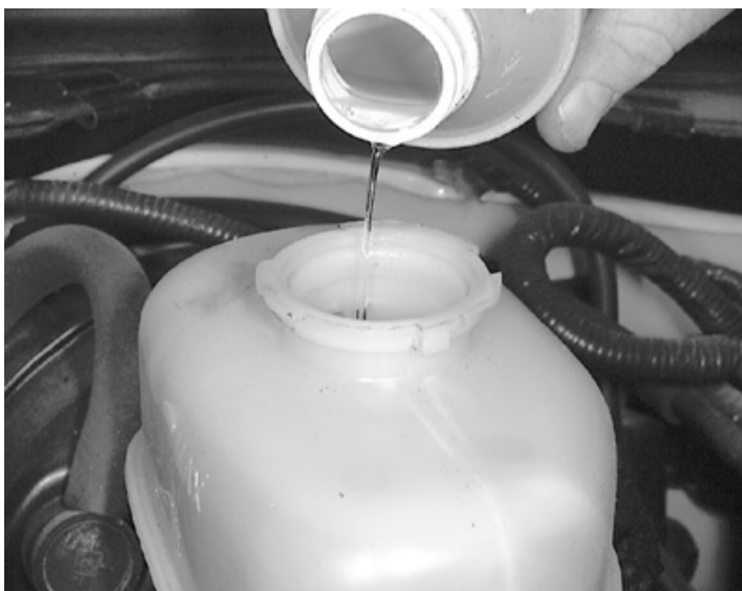
Pour brake fluid from a sealed container directly into the reservoir
