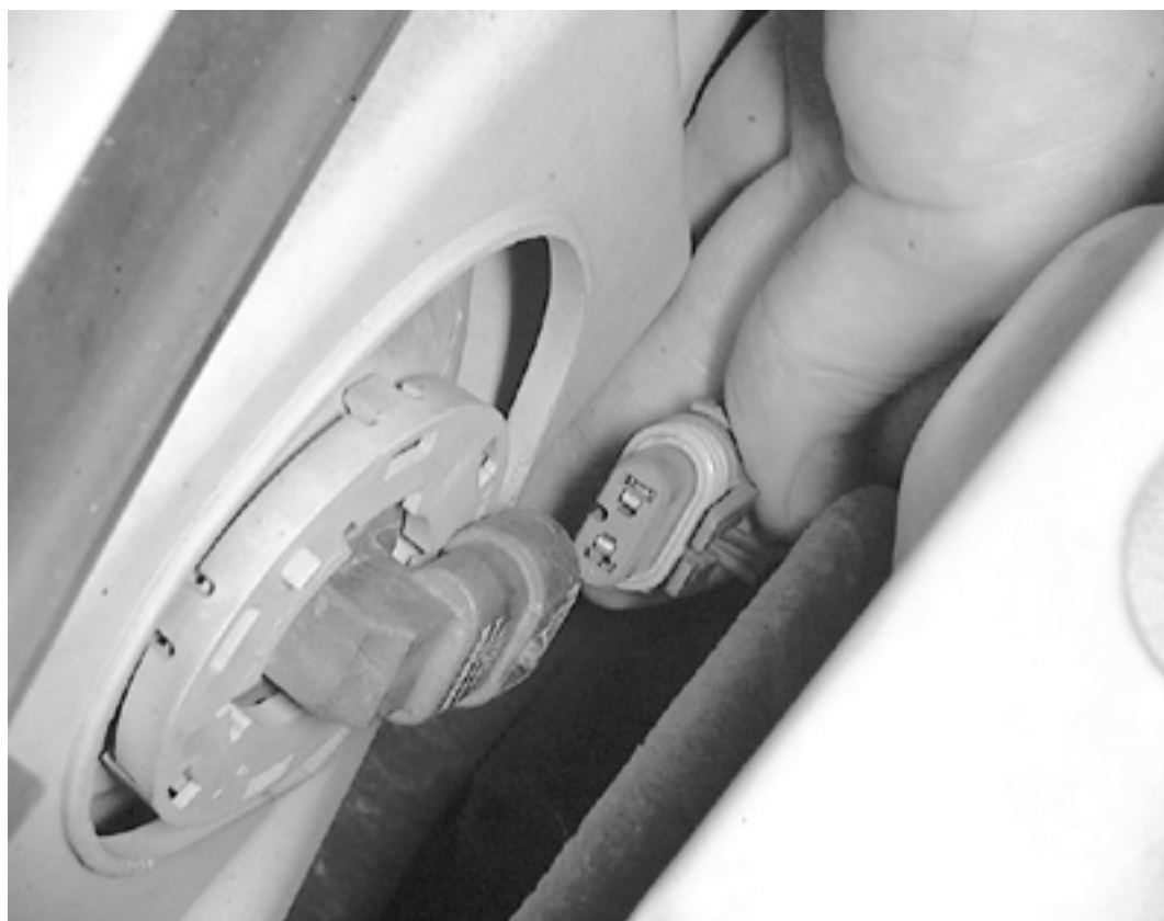
Detach the electrical connector from the bulb
