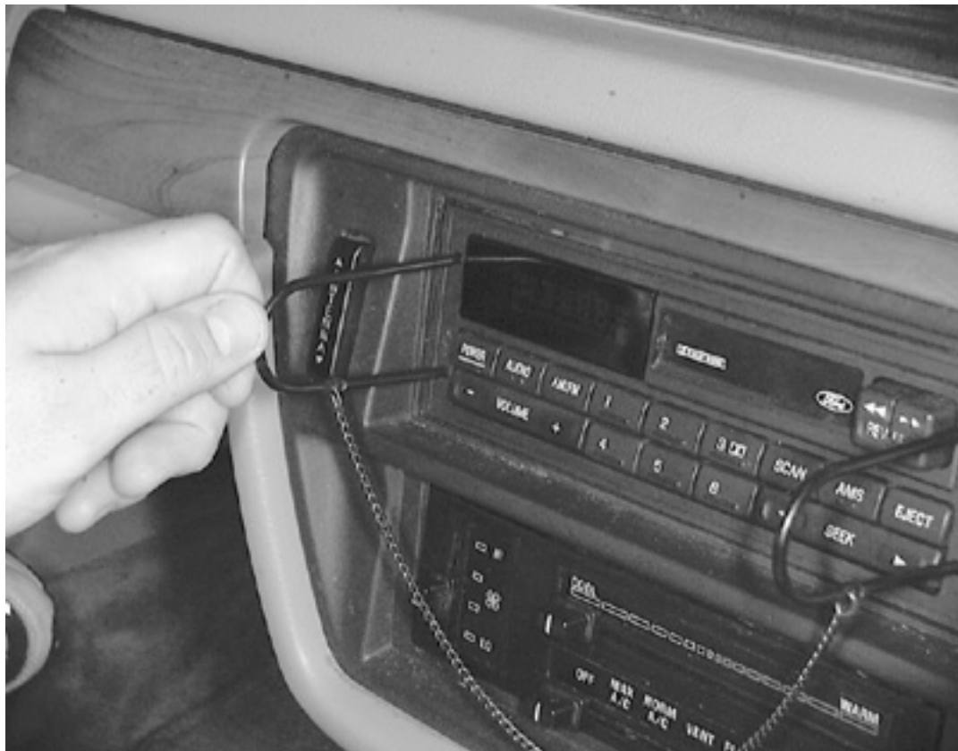
Install Radio Removal Tool (T87P-19061-A) or equivalent into the radio face place
