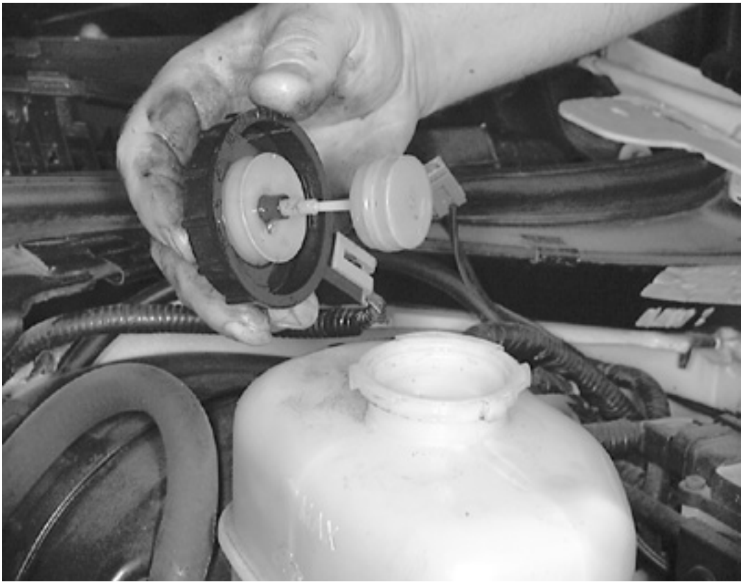
Remove the master cylinder reservoir cap and fluid level sensor
