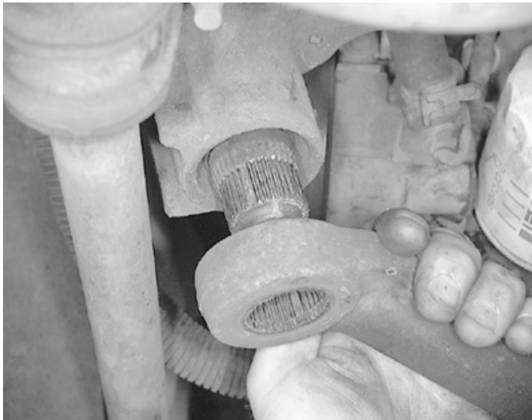
Remove the pitman arm from the steering gear sector shaft
