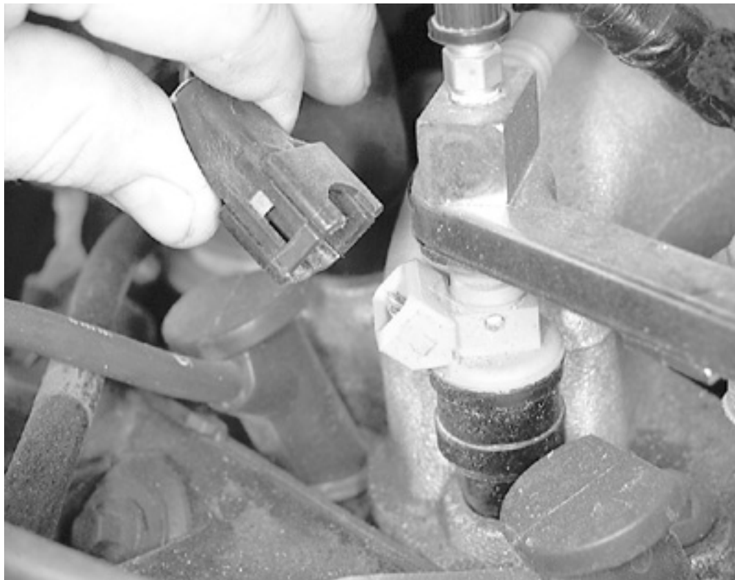
Detach the electrical connectors from the injectors
