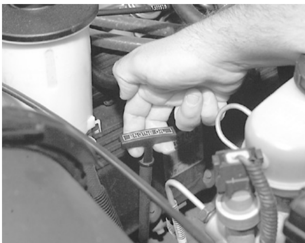
Grasp the engine oil dipstick and ...
