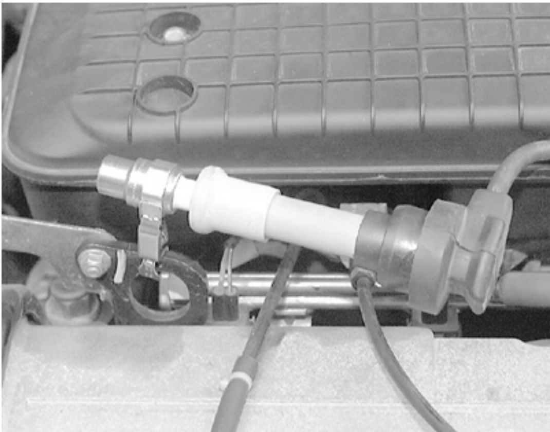
This spark tester looks just like a spark plug, attach the clip to ground and crank the engine to check for spark
