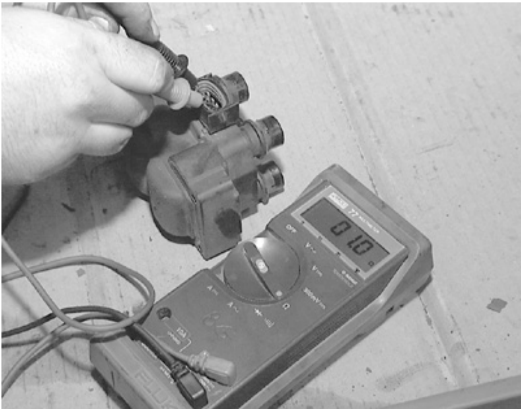
Testing the primary ignition coil resistance-4.6L engine
