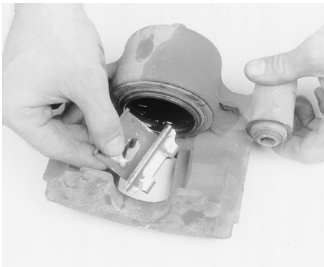
On some vehicles, you must remove the anti-rattle clip
