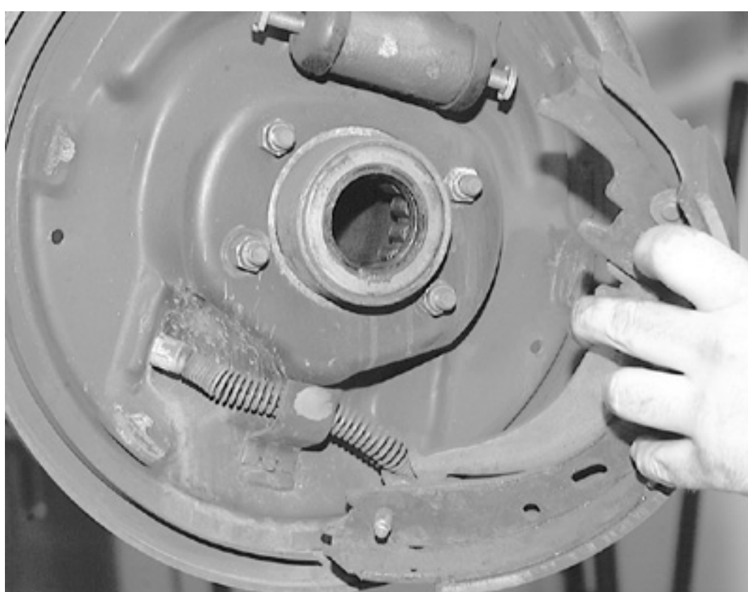
Lift the secondary shoe from the backing plate
