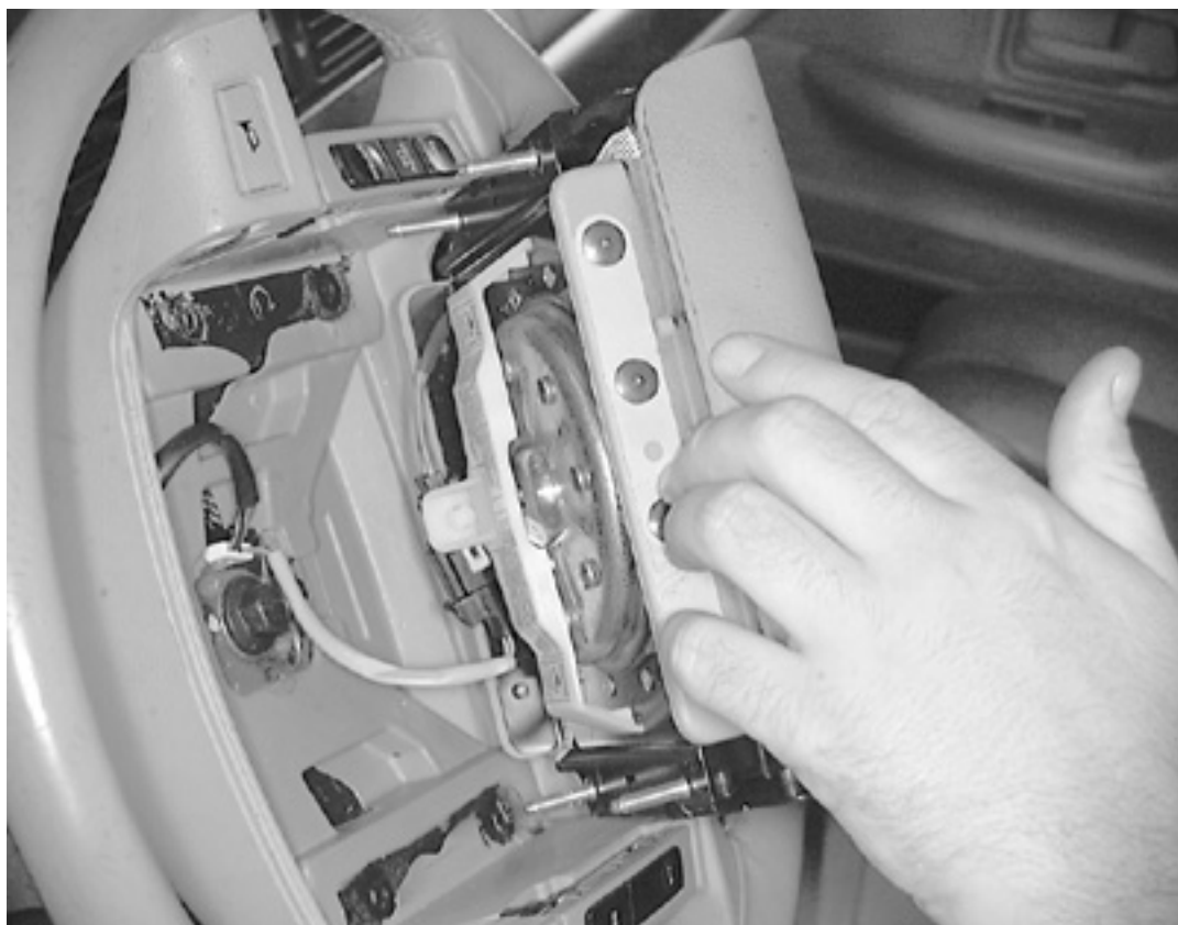
Lift the air bag module from the steering wheel ...
