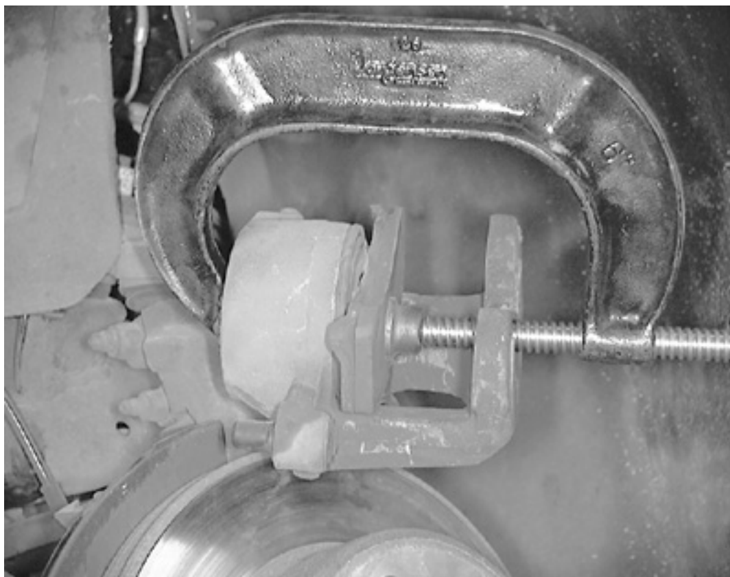
And probably the most popular way is to use a large C-clamp. Just remember to keep the old inner pad in the caliper to keep the piston from being damaged
