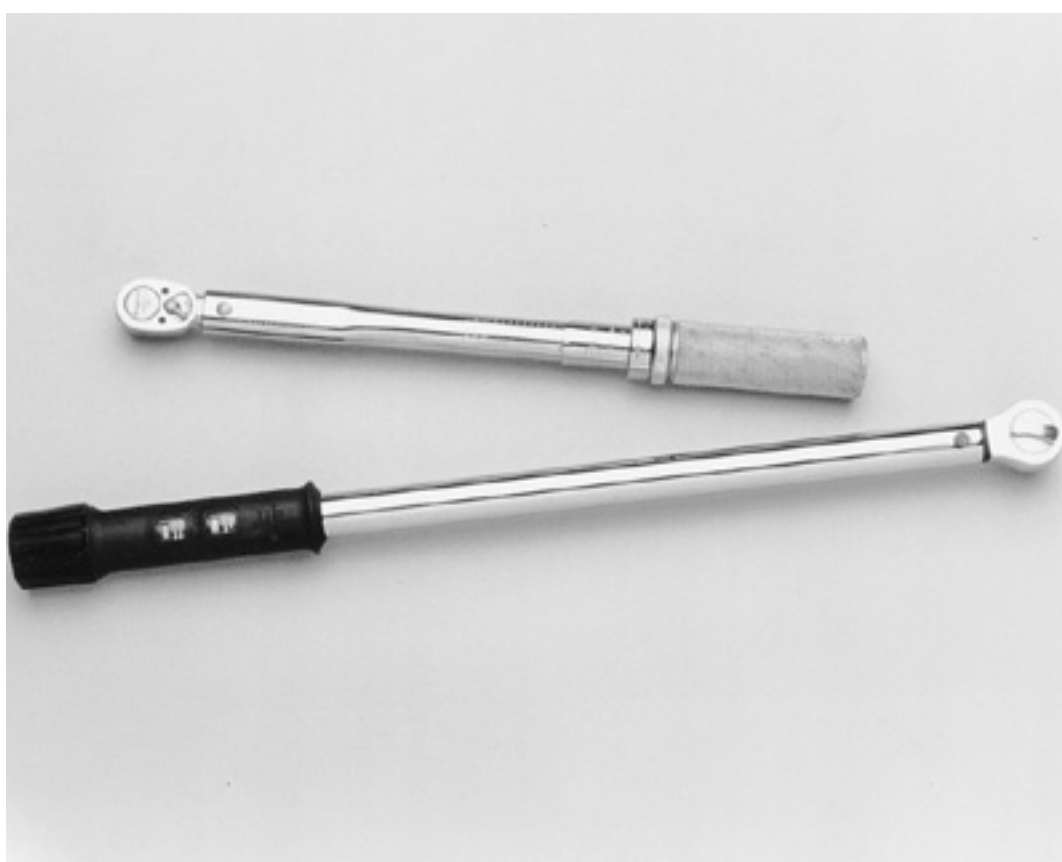
Many repairs will require the use of a torque wrench to assure the components are properly fastened
