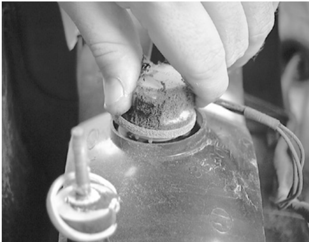
Turn the bulb and socket assembly counterclockwise to remove it from the light assembly to ...
