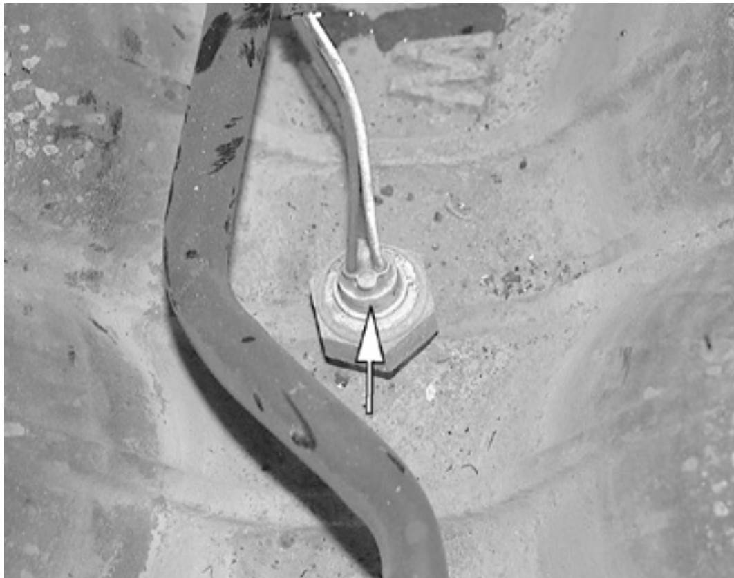
The knock sensor is located under the intake manifold—4.6L Engine
