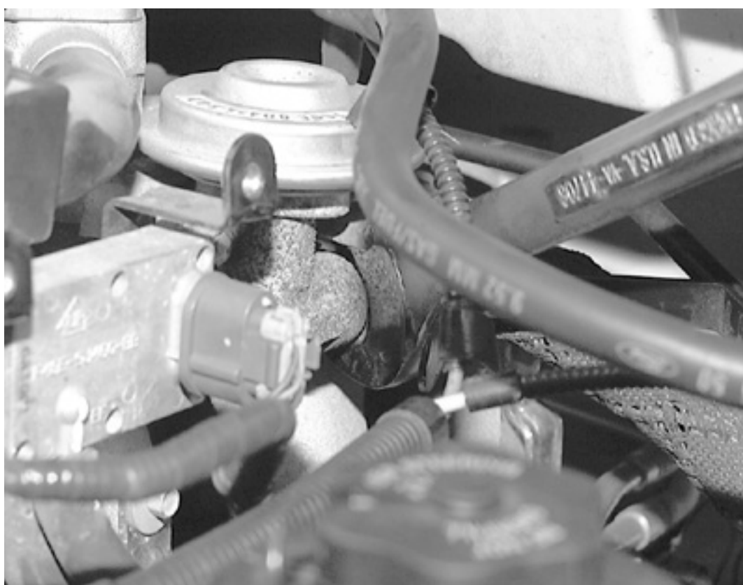
Using a suitable size wrench, loosen the EGR valve-to-exhaust manifold tube and ...
