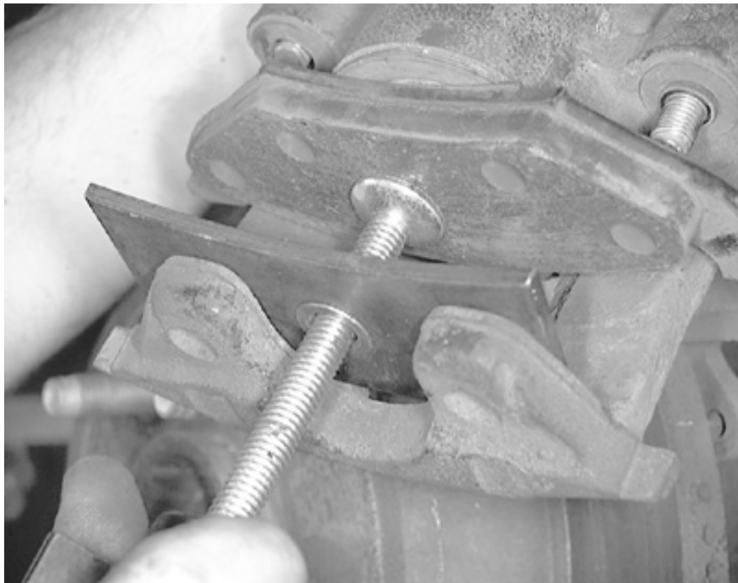
Compress the caliper piston using a suitable special tool or ...
