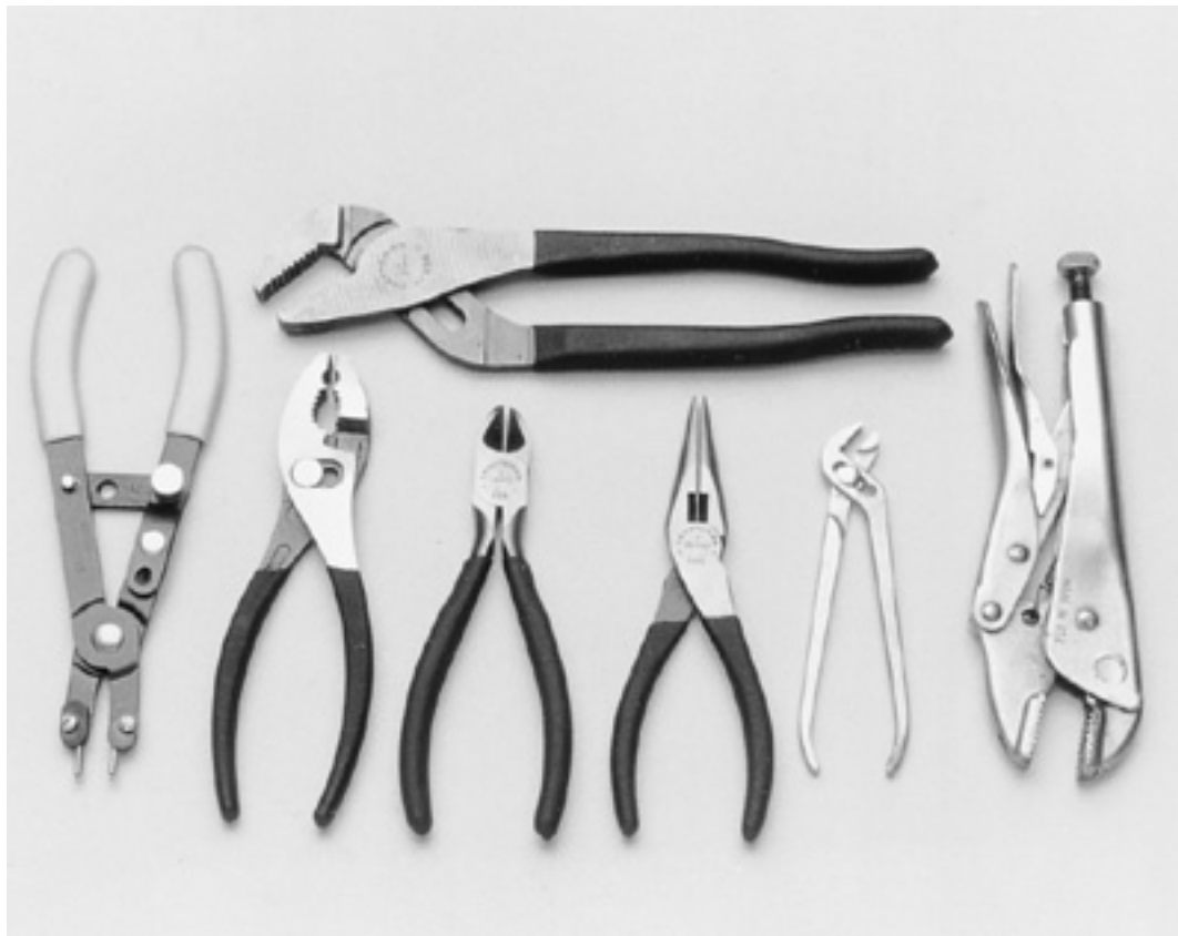
An assortment of pliers, grippers and cutters will be handy for old rusted parts and stripped bolt heads
