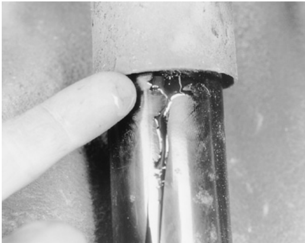
When fluid is seeping out of the shock absorber, it's time to replace it
