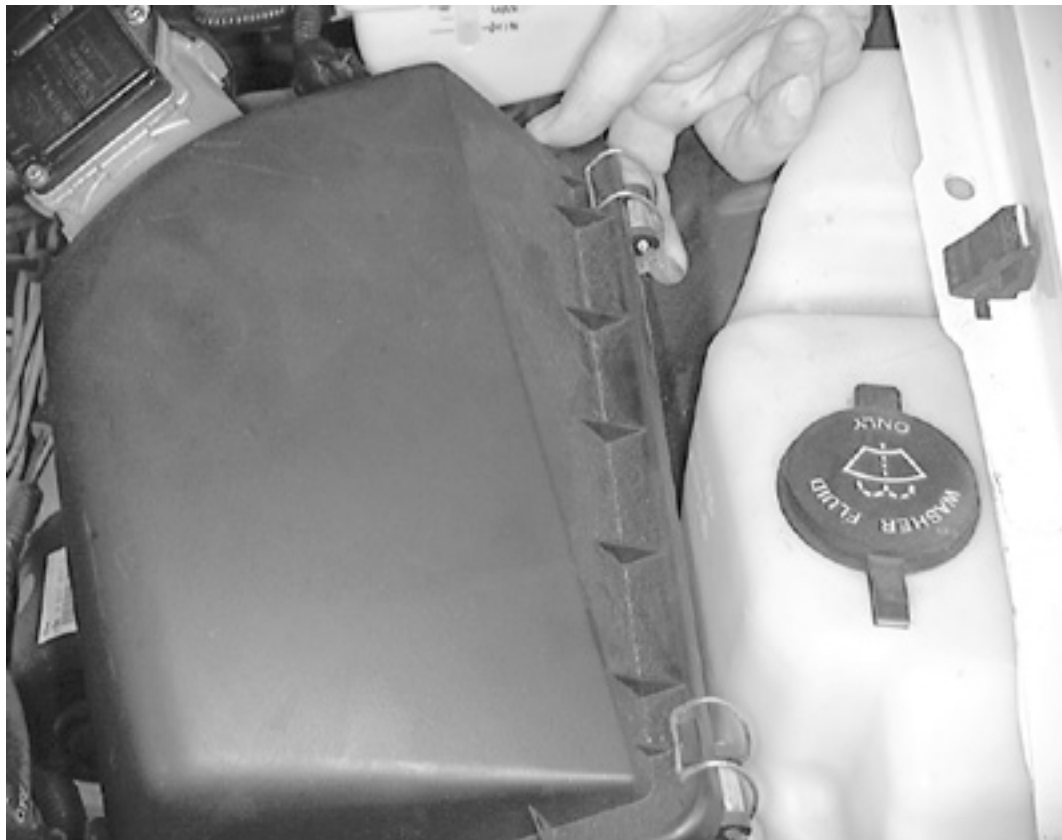
Releasing the spring clips to remove the air cleaner cover—4.6L engine
