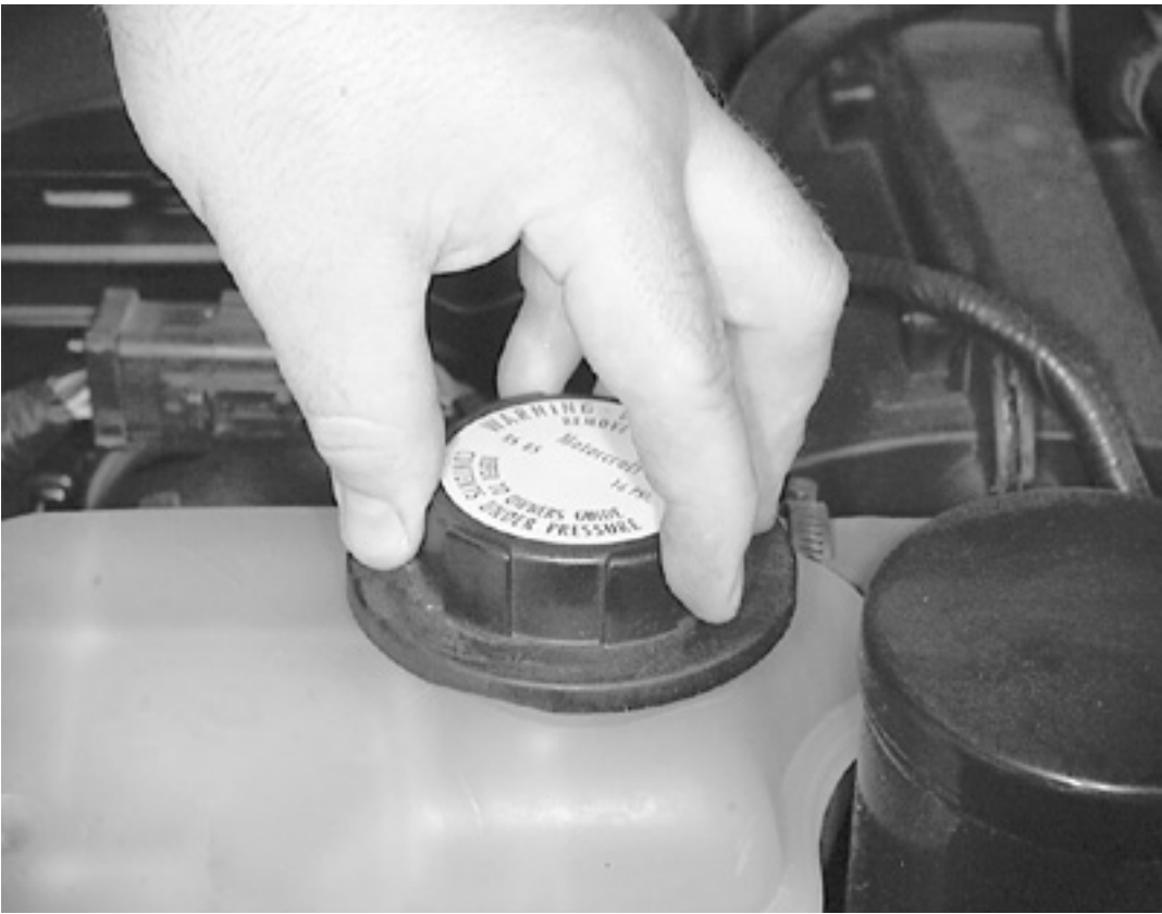
Ensure that the engine is not hot, then loosen the recovery tank cap
