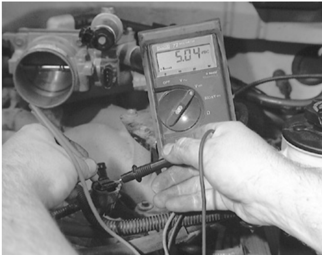
Testing the supply voltage at the TP sensor connector
