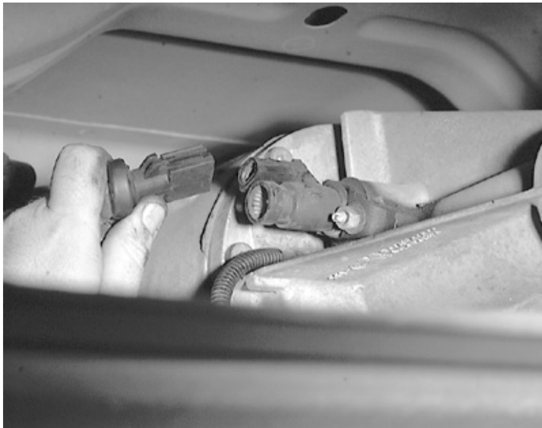
Detach the connector for the VSS sensor
