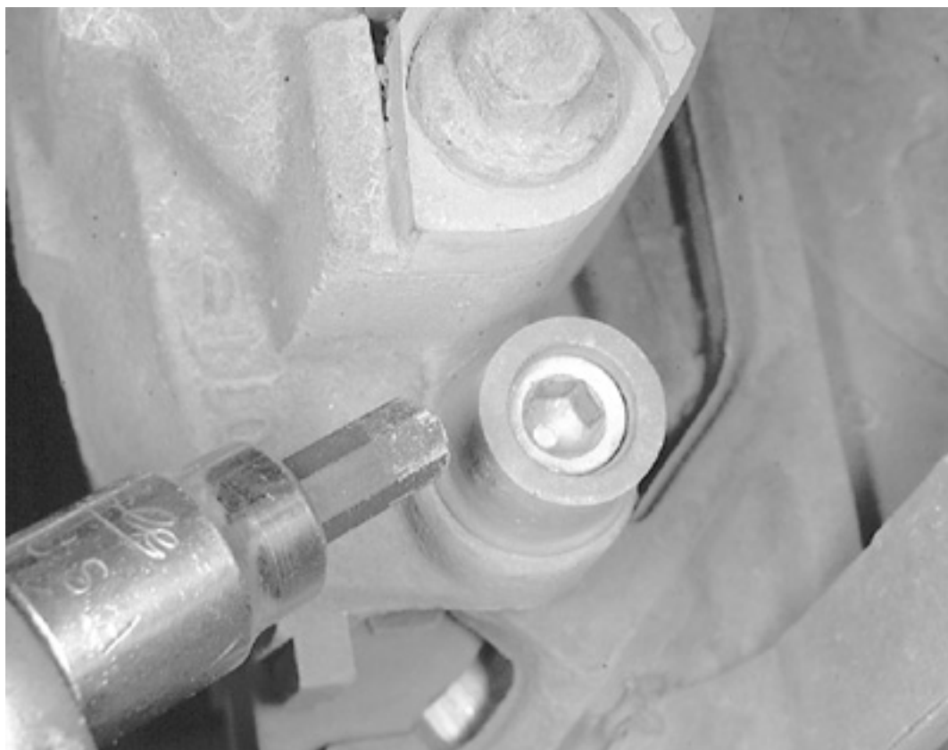
The rear caliper pins typically require a 6mm hex bit
