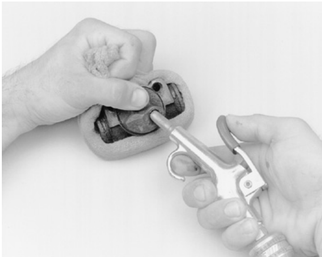
Compressed air can be used to remove the pistons and seals
