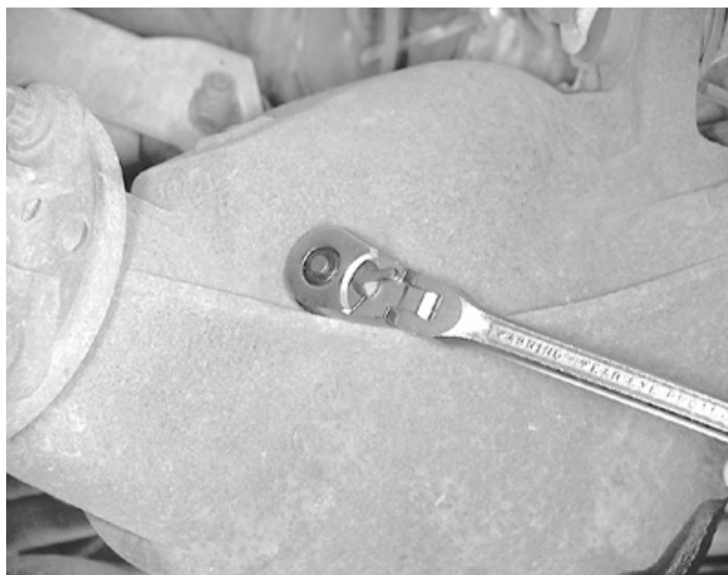
Loosen the check/fill plug with a 3/8 drive tool ...
