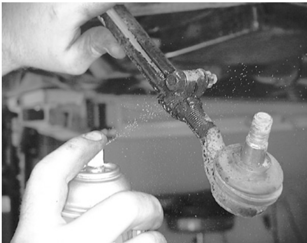
Spraying a quality rust penetrant onto the tie rod adjusting sleeve is a good idea before attempting to remove it
