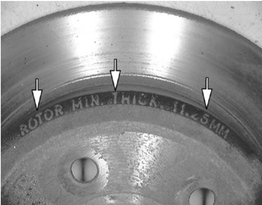
The minimum thickness is typically stamped on the rear rotor in the location shown here
