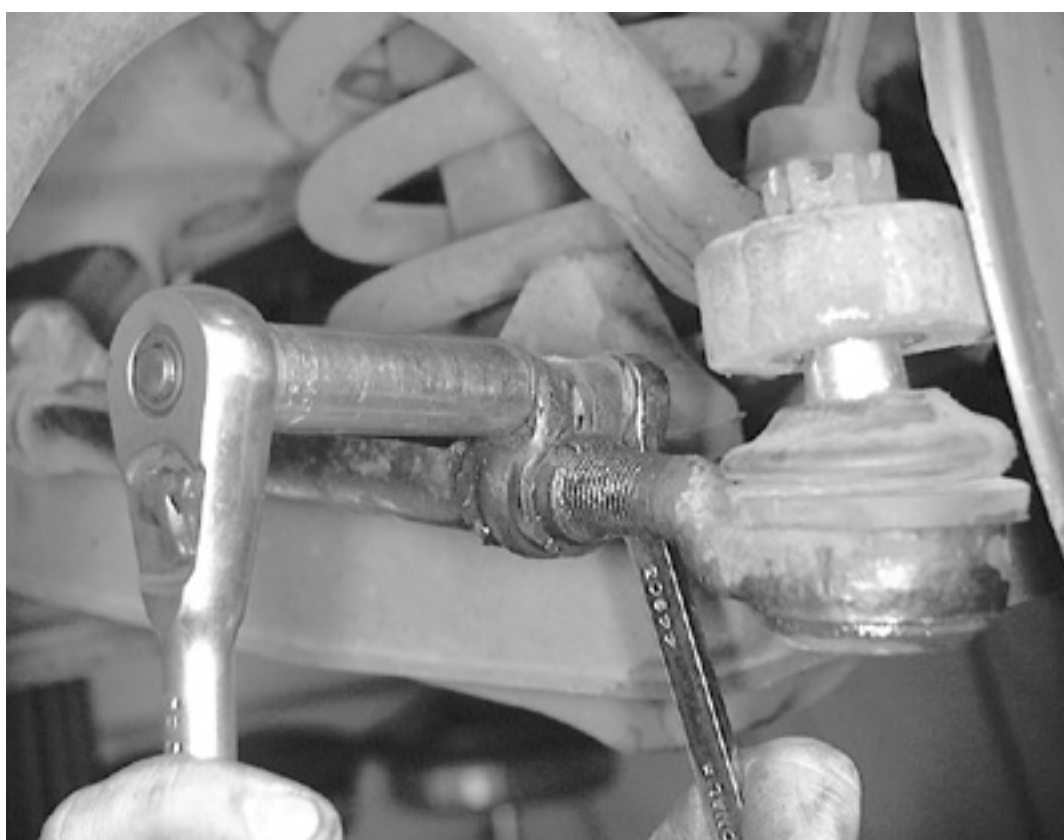
Loosen the adjusting sleeve bolt
