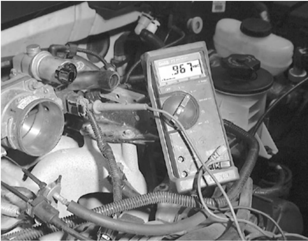
Testing the TP sensor signal return voltage at idle
