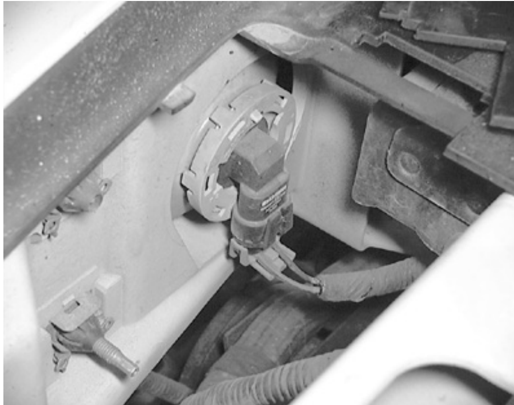
Headlight bulb in installed position
